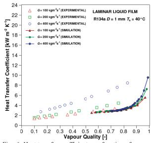
Fig. 6: Heat transfer coefficient as a function of vapour quality. Simulations with laminar liquid film approach and experimental data from Matkovic *et al.* (2009).
