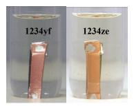
Figure 1: HFO-1234yf and HFO-1234ze with ISO 10 POE oil exposed to 200°C for 2 weeks
