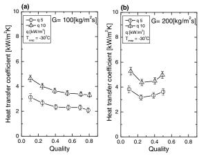
Fig. 6. Heat transfer coefficients at (a) G= 100 kg/m<sup>2</sup>s and (b) G= 200 kg/m<sup>2</sup>s
