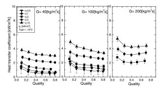
Fig. 2. Heat transfer coefficients with the change of mass and heat fluxes at an evaporation temperature of -15 °C
