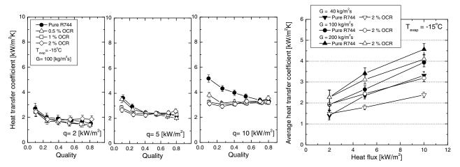
Fig. 9. Effects of oil on the heat transfer coefficient
