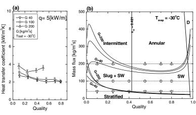
Fig. 4. Average heat transfer coefficients with respect to heat flux
