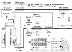
Fig. 1. Simplified schematic of the test facility
