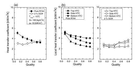
Fig. 11. (a) Heat transfer coefficients and (b) local heat transfer coefficient of pure R744 (left) and oil-R744 mixture of OCR = 2% (right) at evaporation temperature of -15 °C for G = 100 kg/m2s, and q = 10 kW/m2
