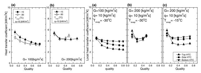
Fig. 7. Effect of evaporation temperature on heat transfer coefficients
