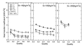
Fig. 3. Heat transfer coefficients with the change of mass and heat fluxes at an evaporation temperature of -30 °C
