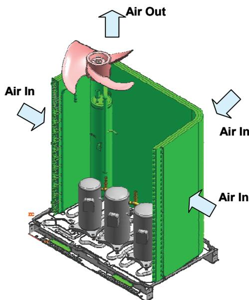
Figure 4 Outdoor chassis structure of large VRF system
