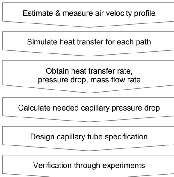
Figure 2 Diagram for design process
