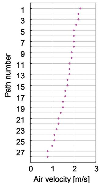
Figure 3 Air velocity profile of VRF outdoor unit
