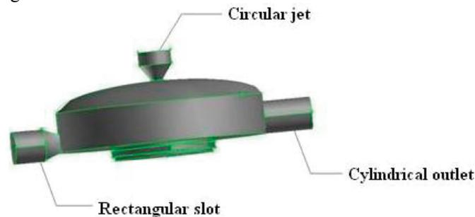
Figure 2: Jet-impingement heat exchanger
