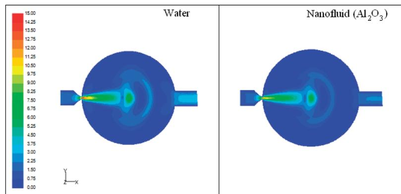
Figure 7: Velocity distribution (m/s) at  $t=15s$  at the mid-plane of the heat exchanger
