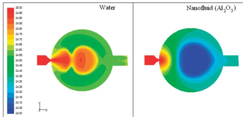
Figure 6: Temperature distribution (°C) at  $t=15s$  at the mid-plane of the heat exchanger
