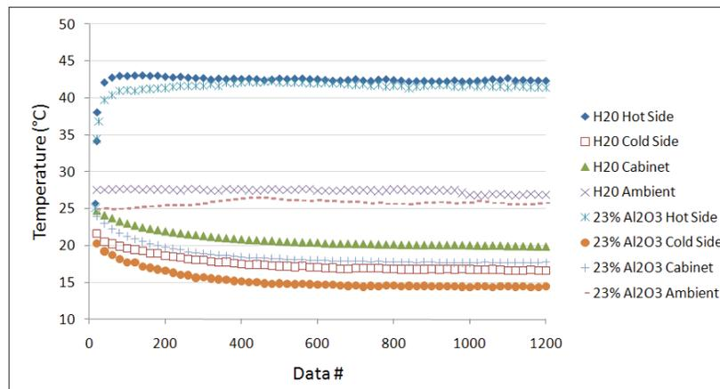
Figure 4: Temperature data from the cooler, cabinet, and ambient
