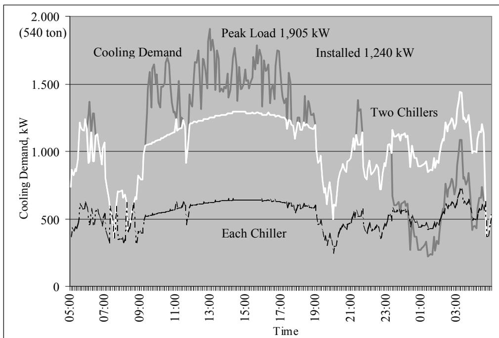
Figure 2: Overall cooling load profile
