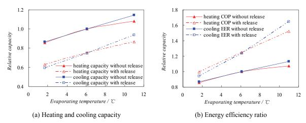
Figure 4. Effect of refrigerant release on the performance of a heat pump system with a scroll compressor
