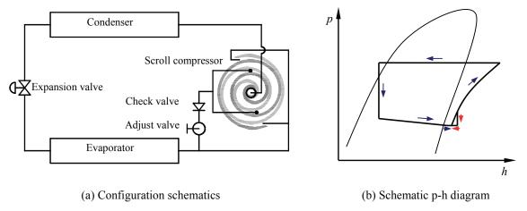
Figure 3. Scroll compressor refrigeration system with refrigerant release
