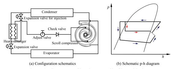
Figure 1. Scroll compressor refrigeration system with refrigerant injection
