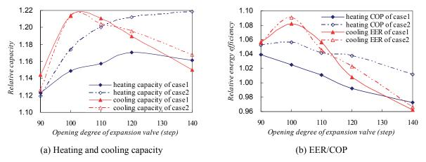
Figure 2. Effect of refrigerant injection on the performance of a heat pump system with a scroll compressor
