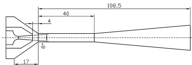
Figure 3: Axi-symmetric cross-section of tested ejector
