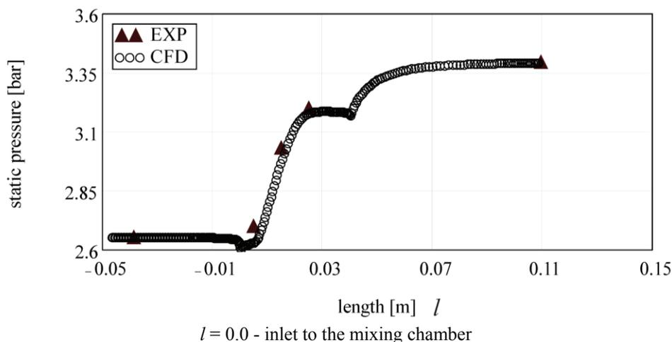
Figure 5: Comparison of calculated static pressure profile with experimental data
