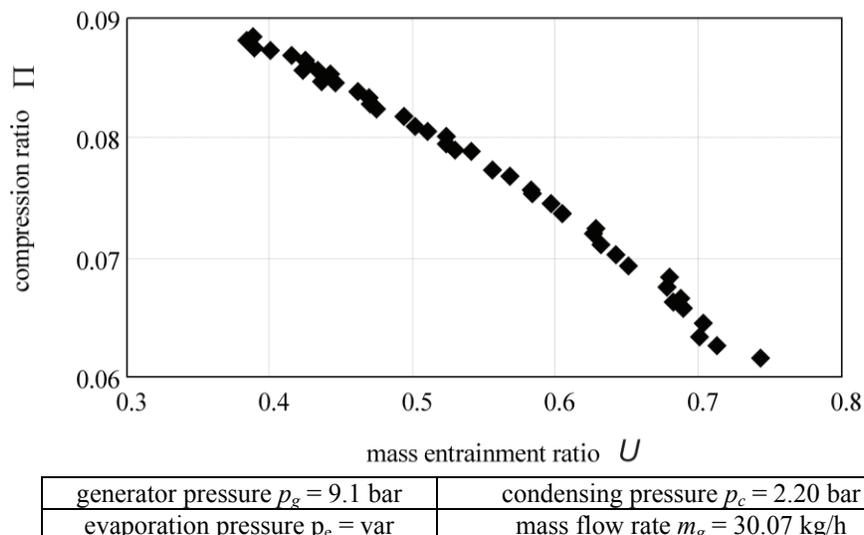
Figure 4: Experimental compression ratio  $\Pi$  versus mass entrainment ratio  $U$ .
