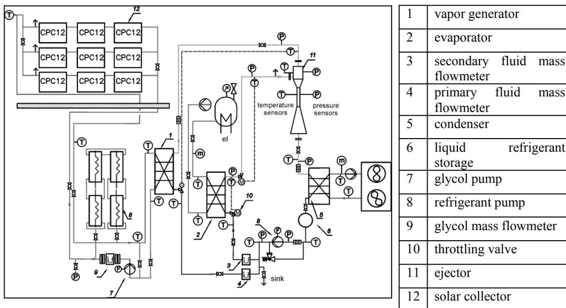
Figure 2: Schematic of the testing rig.
