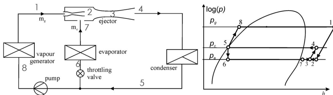
Figure 1: Schematic diagram of ejector device and ejector cycle in  $\log(p)$ - $h$  co-ordinates
