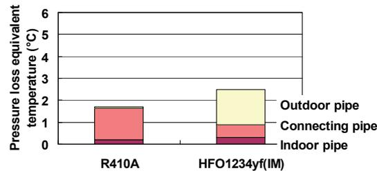
Figure 8: Pressure loss breakdowns between evaporator outlet and compressor inlet
