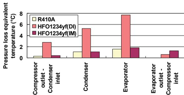
Figure 4: Pressure loss characteristics at rated heating capacity
