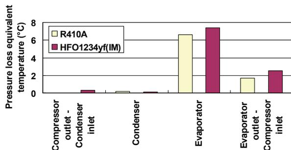
Figure 6: Pressure loss characteristics at rated cooling capacity
