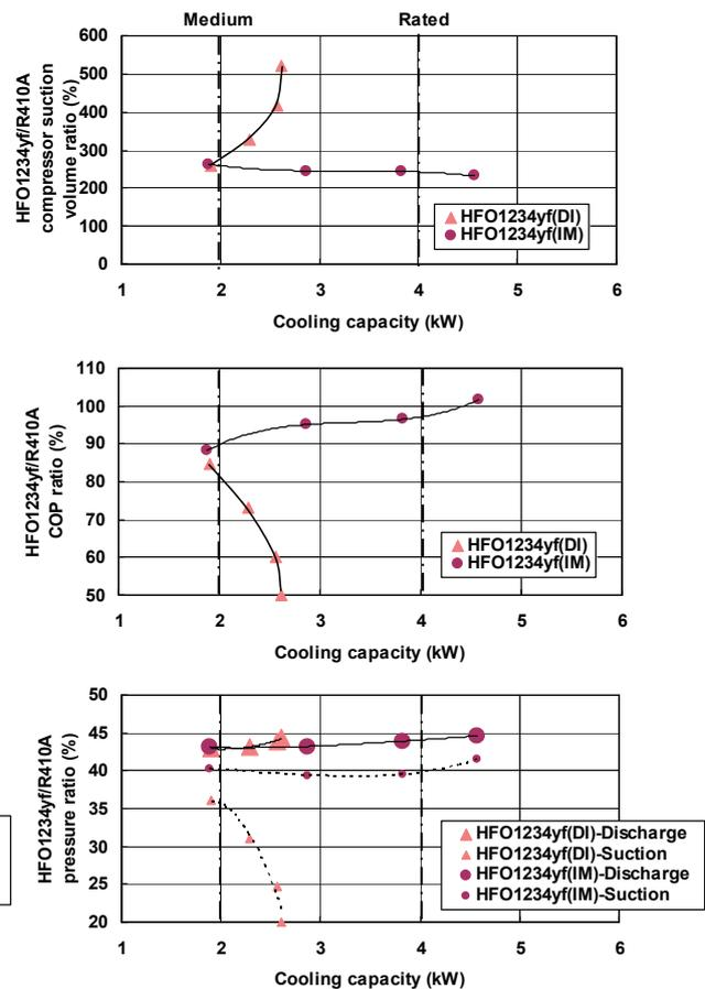
Figure 3: Cycle performance characteristics in cooling operation
