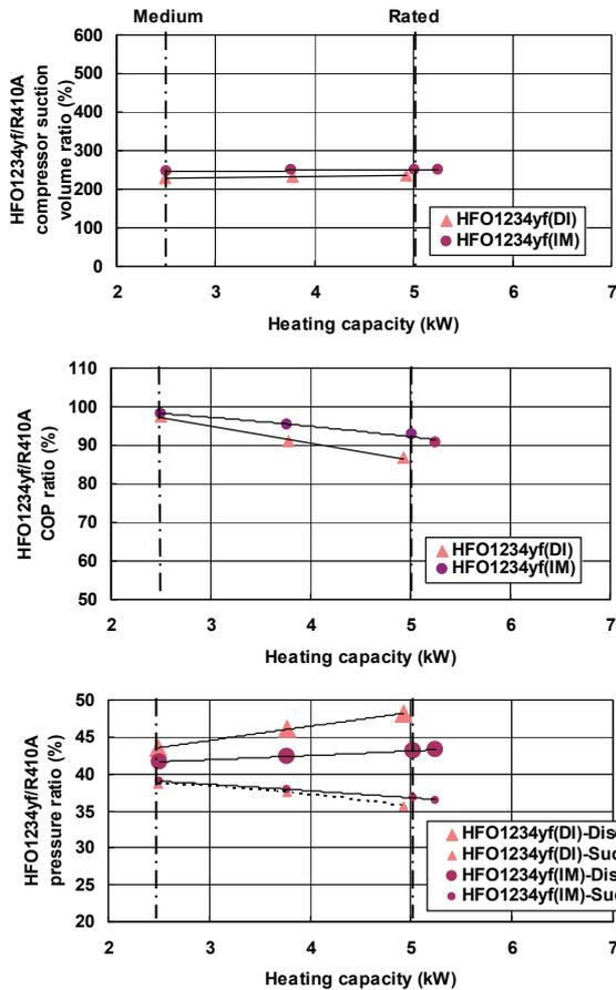
Figure 2: Cycle performance characteristics in heating operation
