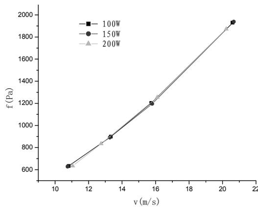
Figure 8 : Pressure drop VS. flowing velocity for helium
