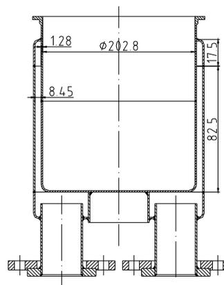
Figure 4 : NMC in the simulating experiment
