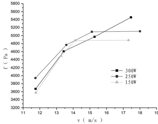
Figure 6 Pressure drop VS. Flowing velocity for Nitrogen
