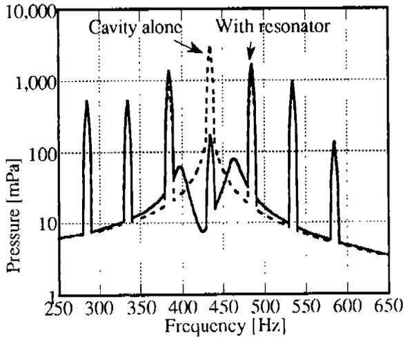
Figure 8: Simulation of experimental results, one mode in the model
