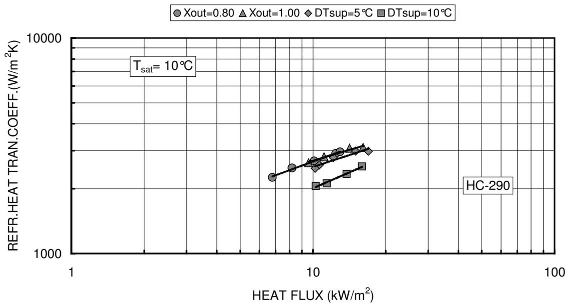
Figure 3: Average heat transfer coefficient on refrigerant side vs. heat flux at 10°C of saturation temperature
