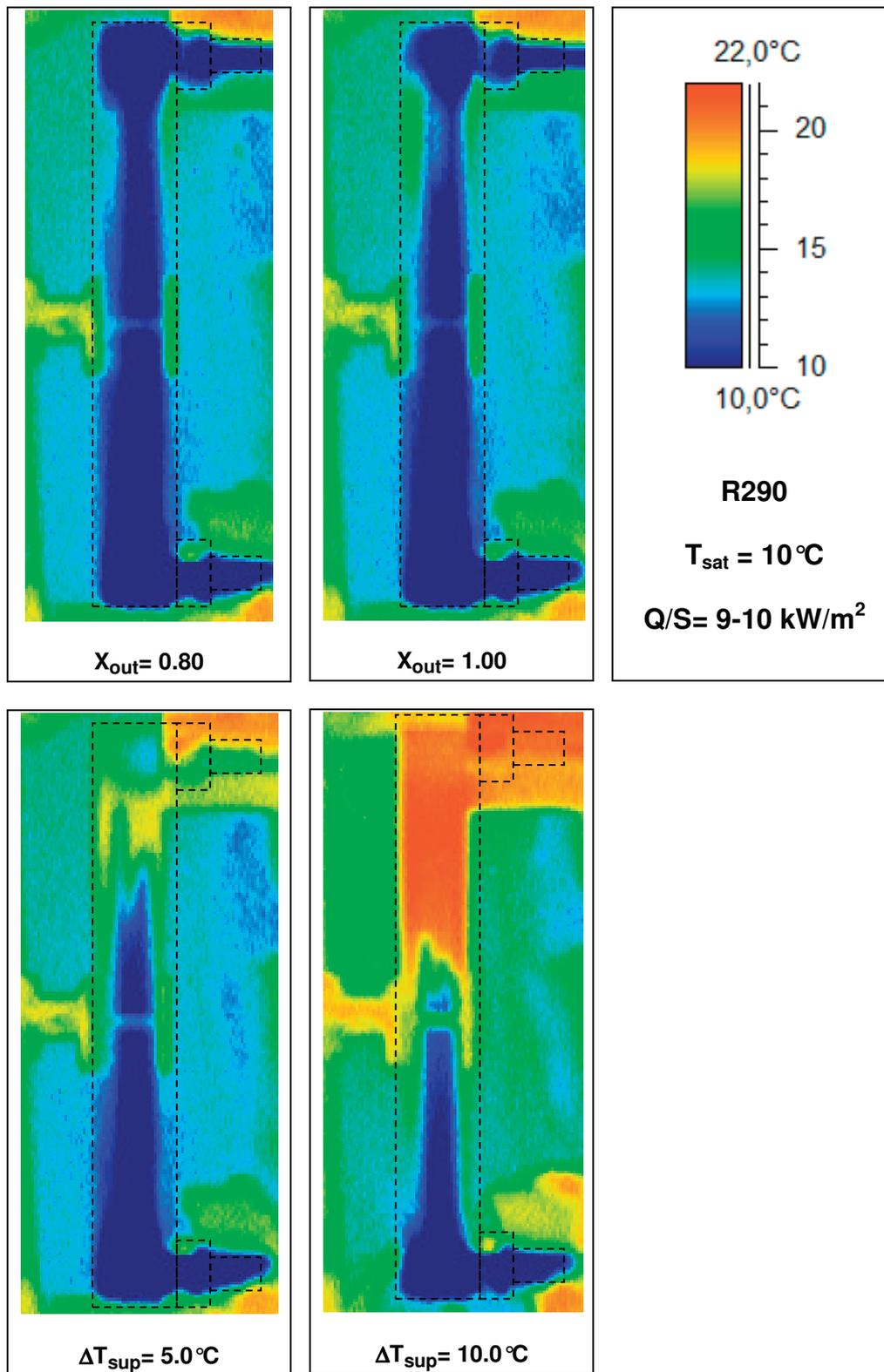
Figure 7: IR thermography of the BPHE during HC-290 vaporisation tests at  $10^\circ\text{C}$  of saturation temperature with a heat flux around  $9-10 \text{ kW/m}^2$  and different evaporator outlet conditions
