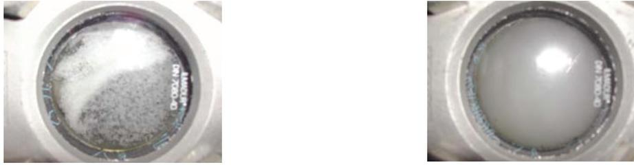
Figure 2: Appearance of CO<sub>2</sub> hydrate slurry.
