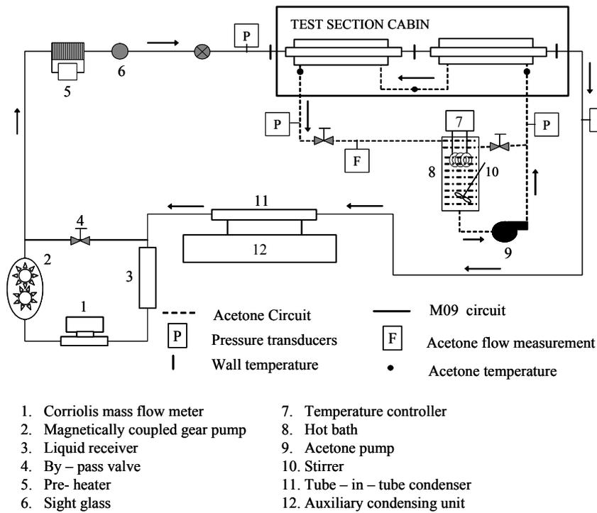
Figure 1 Schematic view of the Experimental setup
