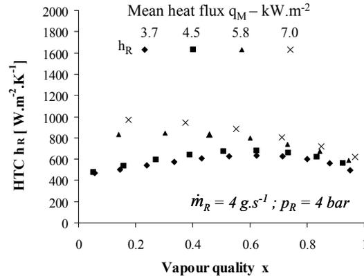
Figure 3: Influence of mean flux on heat transfer coefficient at 4 bar
