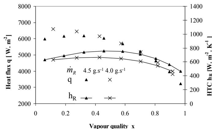
Figure 2 : Variation of heat flux with respect to dryness fraction
