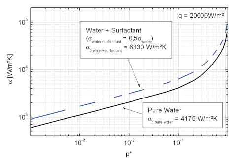
Figure 6: Possible increase of the heat transfer coefficient  $\alpha$  by halving the surface tension  $\sigma$ . The predictions are calculated according to Gorenflo (1984) and Kotthoff/Gorenflo (2005)
