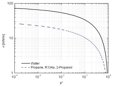
Figure 3: Comparison of the surface tension of water, propane, R134a and 2-propanol at the respective saturation temperature
