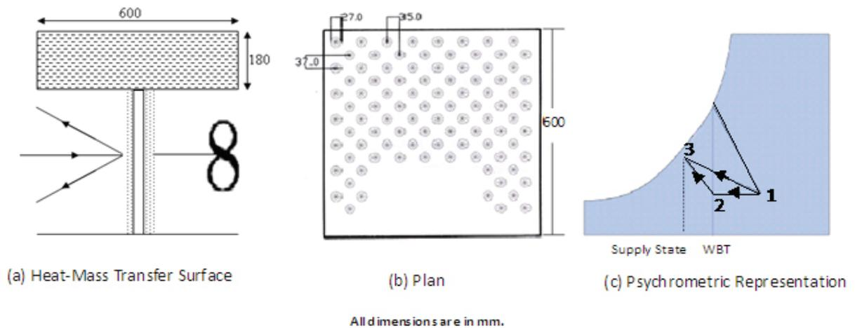
Fig 2. Design of the proposed SIEC
