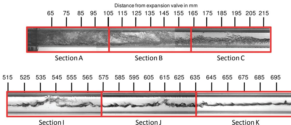
Flow Conditions: ID = 8.7mm, mass flux =  $336 \text{ kg/m}^2\text{s}$ , quality = 15%
