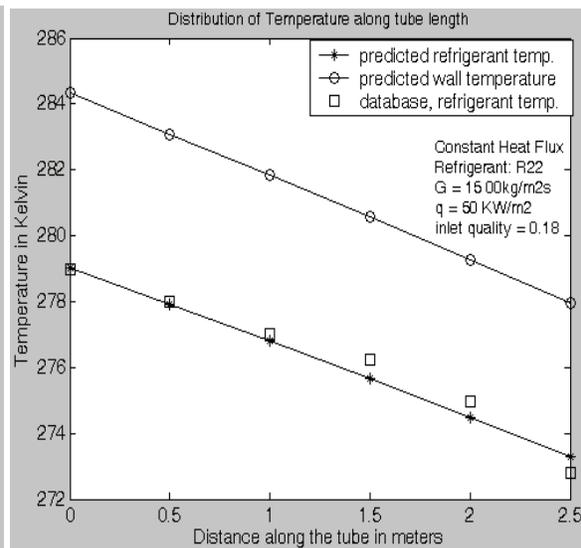
Figure 2b: Temperature distribution along tube length
