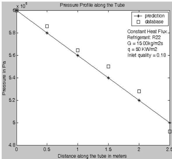
Figure 2a: Pressure distribution along tube length
