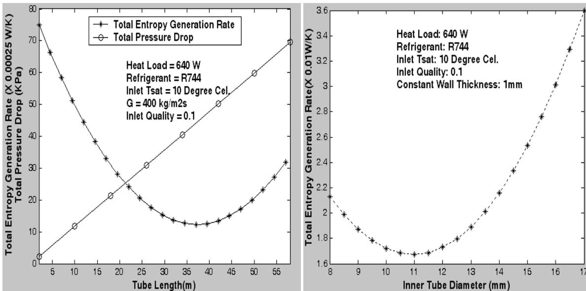
Figure 3a: Entropy generation rate for varying tube length Figure 3b: Entropy generation rate for varying diameter
