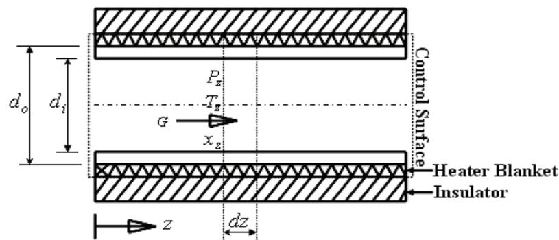
Figure 1: The Tube Model
