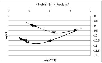
Figure 9: Entropy generation profile for two design points from problem A and problem B
