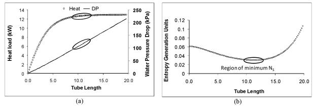
Figure 3: Effect of varying tube length for hot water coil on entropy generation, heat load and refrigerant pressure drop
