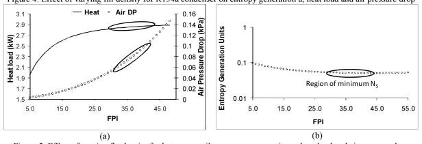
Figure 5: Effect of varying fin density for hot water coil on entropy generation a, heat load and air pressure drop
