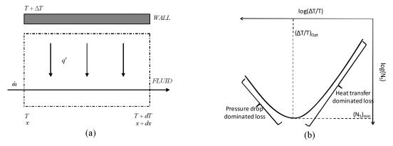
Figure 1: Schematic of entropy generation and optimum point of operation.
