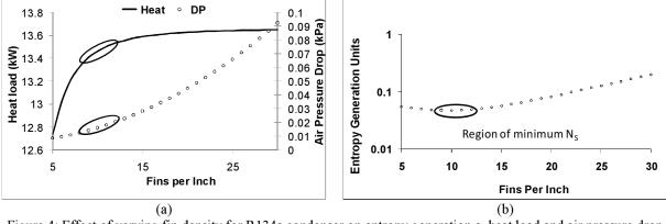
Figure 4: Effect of varying fin density for R134a condenser on entropy generation a, heat load and air pressure drop
