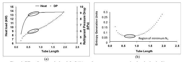
Figure 2: Effect of varying tube length for R134a condenser on entropy generation, heat load and refrigerant pressure drop
