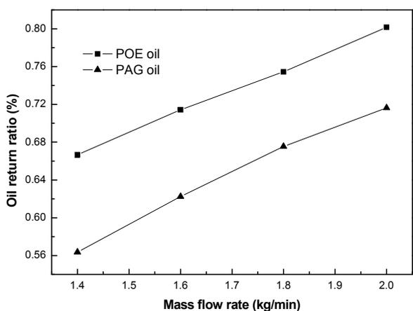
Fig. 9 Effect of the mass flow rate on PAG and POE oils return ratio at 10 °C, 3 wt.%
