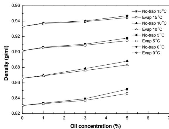
Fig. 6 Density of CO2/POE oil mixture for oil concentration and temperature
