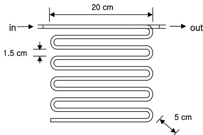
The coolant flow loop contains a constant-temperature bath, a cooler and a water pump. The temperature of CO<sub>2</sub>/oil mixture can be controlled by the temperature of Ethylene Glycol/Water in the cooler and the flow rate. Fig. 2 shows the details of an evaporator model, which was made of stainless steel to endure the high pressure and insulated to minimize heat loss. The diameter of the evaporator tube is 1/4 inch.
