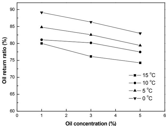
Fig. 7 Effect of the oil concentration on POE oil return ratio
