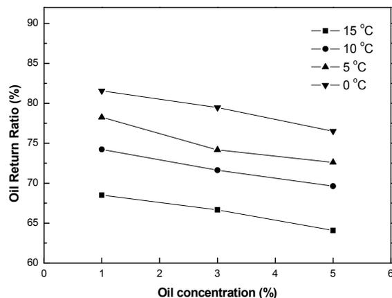
Fig. 4 Effect of the oil concentration on PAG oil return ratio
