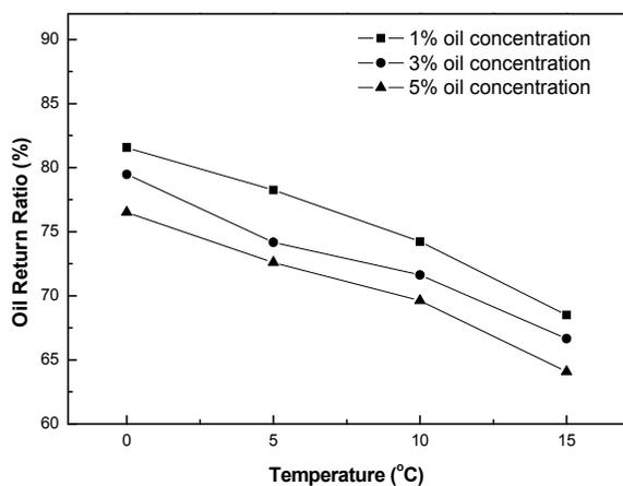
Fig. 5 Effect of the temperature on PAG oil return ratio
