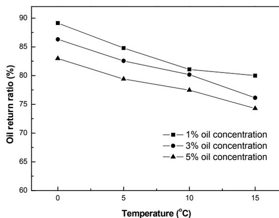
Fig. 8 Effect of the temperature on POE oil return ratio
