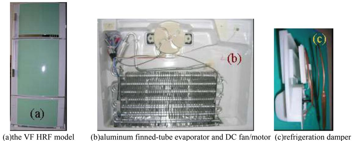
Figure 2: Photos for the VF HRF System and components in this study
