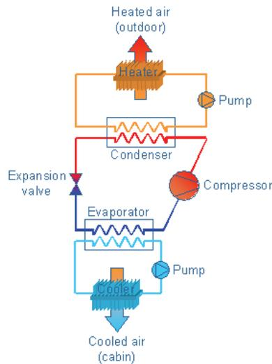
Figure 1: Indirect air-conditioning primary and secondary loops
