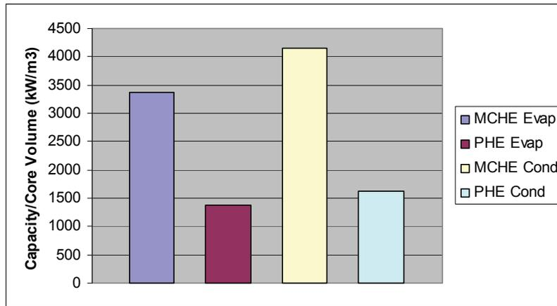
Figure 3: Comparison of the volumetric capacity of MCHE and PHE (Shiba *et al.* 2007).
