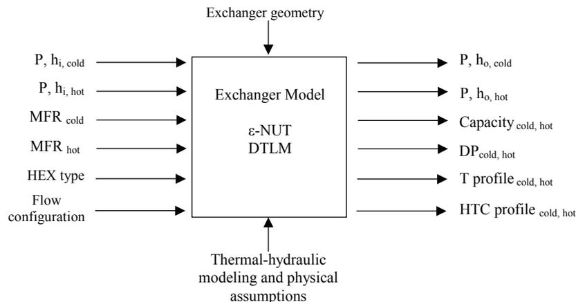
Figure 2 : Heat Exchanger model inputs and outputs.
