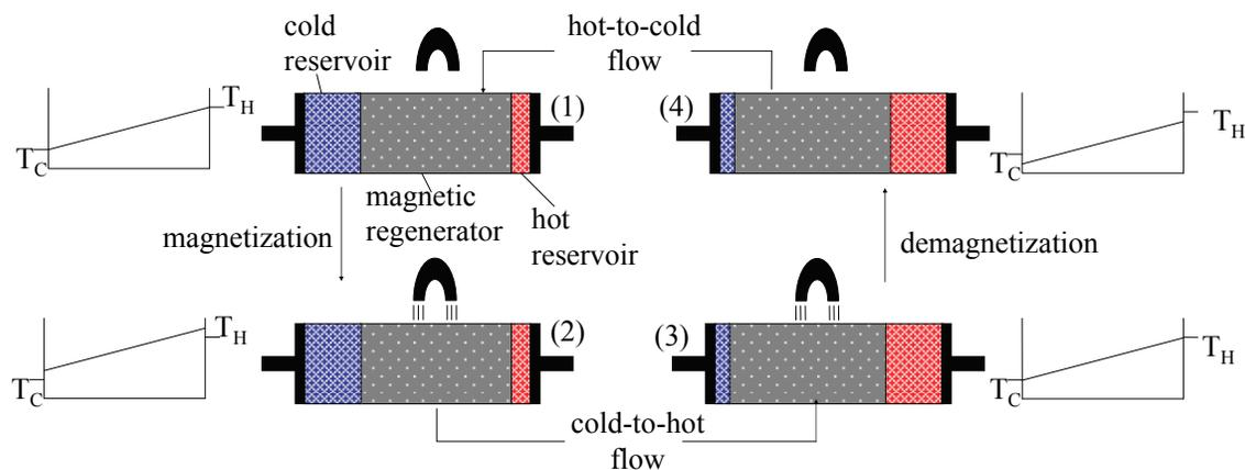
Figure 2: Active Magnetic Regenerative Refrigeration Cycle
