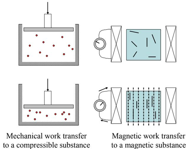
Figure 1: Analogy between magnetic work and mechanical work
