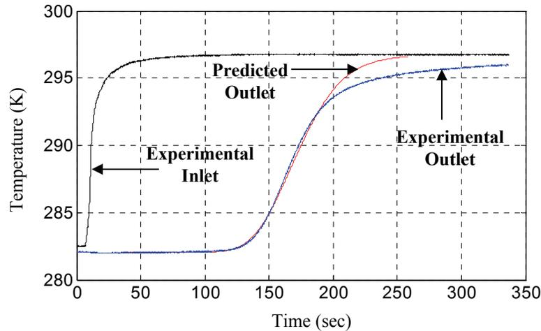
Figure 7: Experimental inlet, outlet, and model predicted temperatures as a function of time
