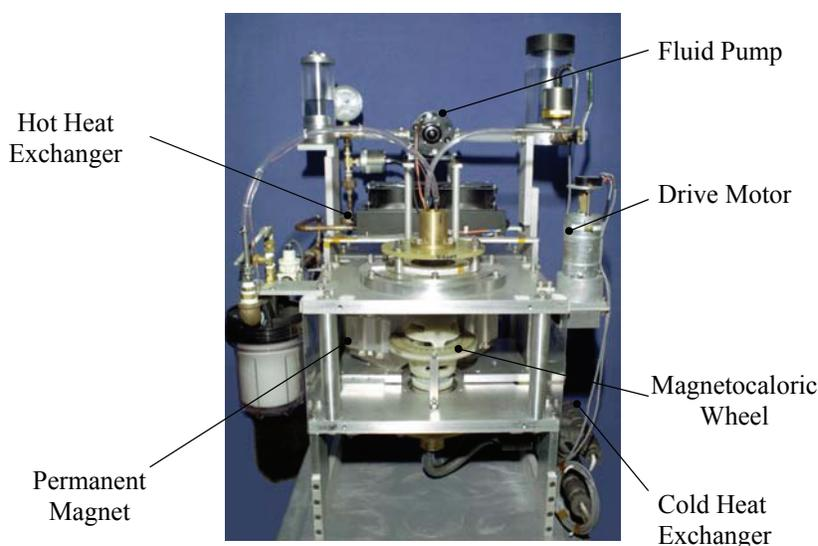
Figure 3: Rotary AMRR experiment at Astronautics
