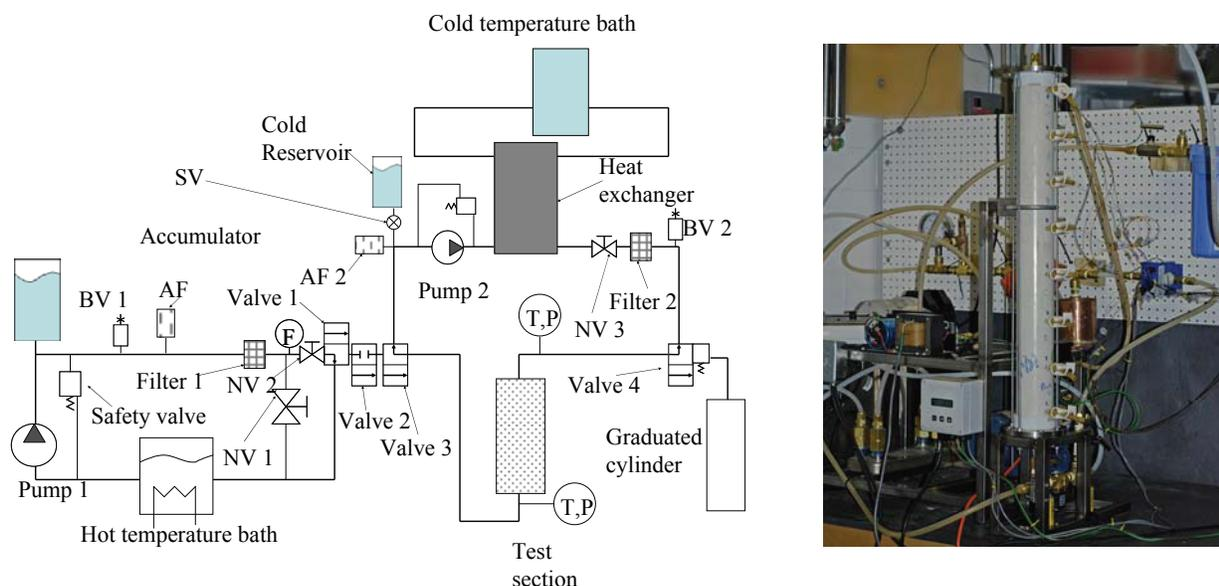
Figure 6: Flow schematic (left) and photograph (right) of the regenerator test facility
