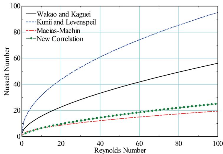
Figure 5: Nusselt number correlations from literature and the newly developed correlation from section 3.2, with a Prandtl number of 30 and porosity of 0.36
