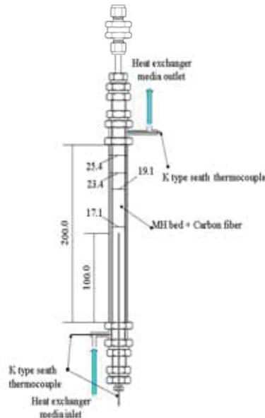
Figure 4 : Heat exchanger of MH2
