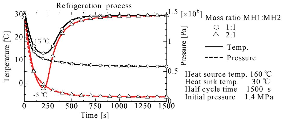
Figure 8 : Temperature and pressure change history at different MH mass ratio
