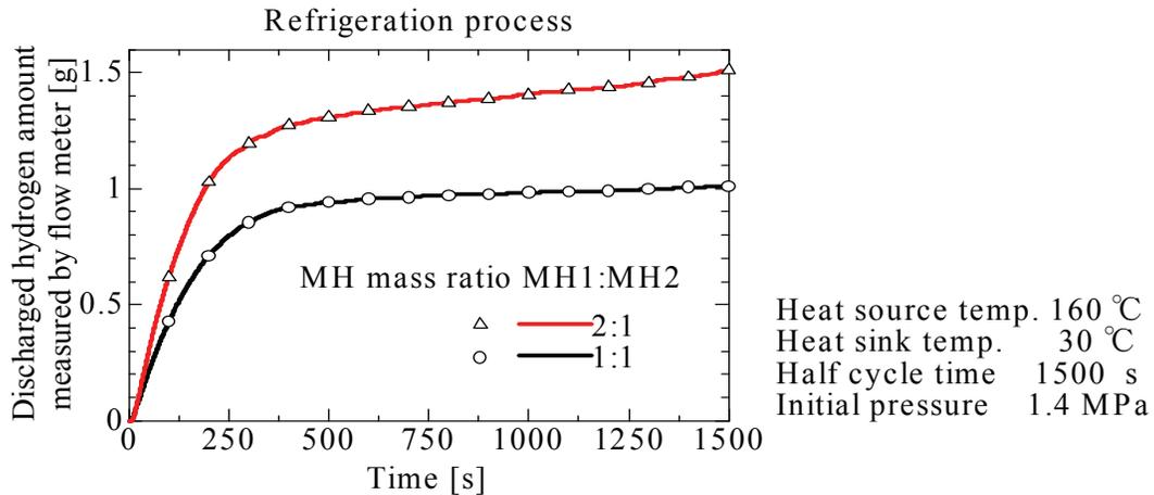
Figure 7 : Discharged hydrogen amount of MH2 at different MH mass ratio
