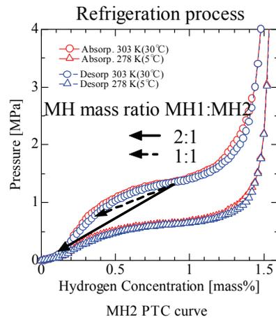
Figure 9 : Condition change of MH2 at different MH mass ratio
