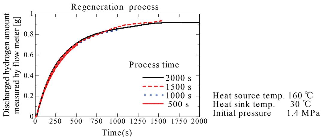
Figure 5 : Influence of regeneration process time on the discharged hydrogen amount of MH2
