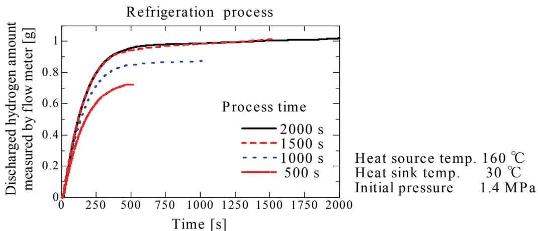
Figure 6 : Influence of refrigeration process time on the discharged hydrogen amount of MH2
