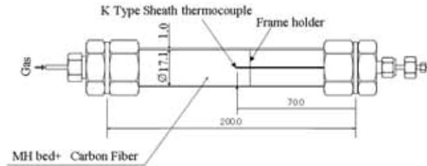
Figure 3 : Heat exchanger of MH1
