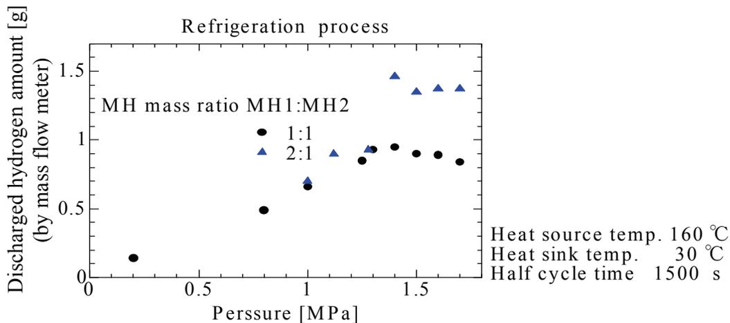
Figure 10 : Initial hydrogen supplying pressure vs. discharged hydrogen amount of MH2
