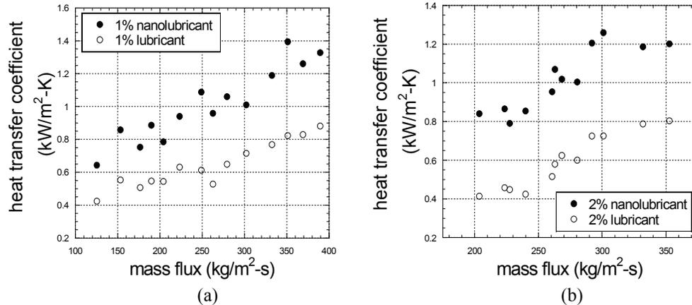
Figure 6: Heat transfer enhancement as a function of mass flux for (a) 1% nanolubricant and (b) 2% nanolubricant
