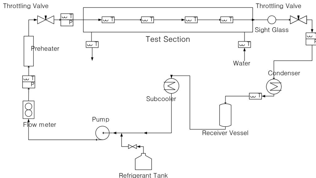
Figure 2: Schematic of the experimental apparatus
