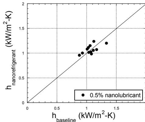
Figure 4: A mass fraction of 0.5% nanolubricant has no apparent effect on the evaporative heat transfer coefficient of R-134a
