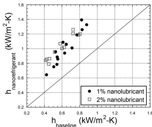
Figure 5: Mass fractions of 1% and 2% nanolubricant increase the evaporative heat transfer coefficient of R-134a
