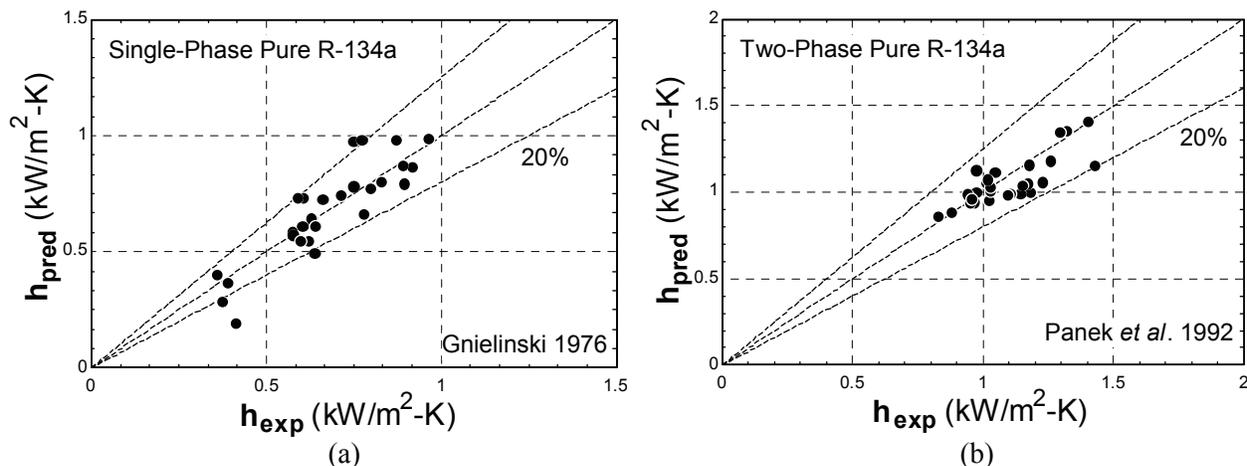
Figure 3: Comparison of experimental data to (a) Gnielinski's correlation for the single-phase-flow data, and (b) Panek's model for the flow-boiling data
