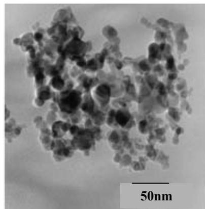
Figure 1: Copper (II) oxide nanoparticles (average size ~ 30 nm). Image from Nanophase Technologies Corp.
