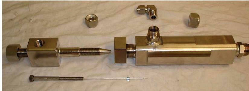
Figure 5: Photograph of controllable ejector expansion device
