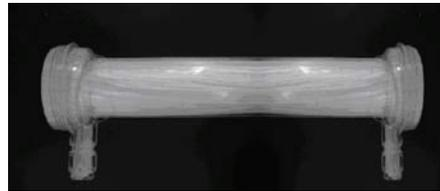
Fig.1. Hollow fiber membrane heat exchanger module
