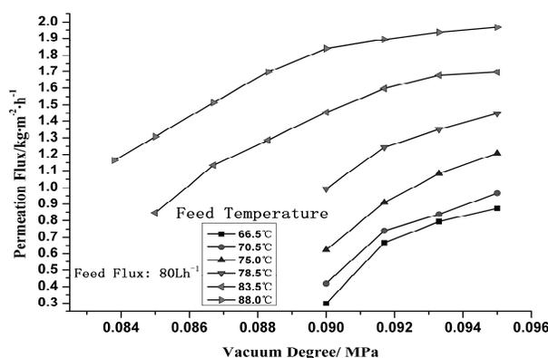
Fig.6 Influence of vacuum degree on permeation flux
