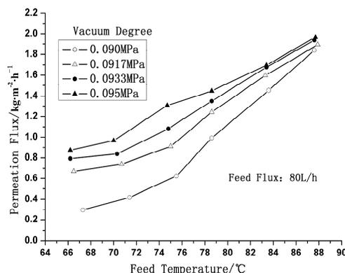
Fig.4 Influence of feed temperature on permeation flux
