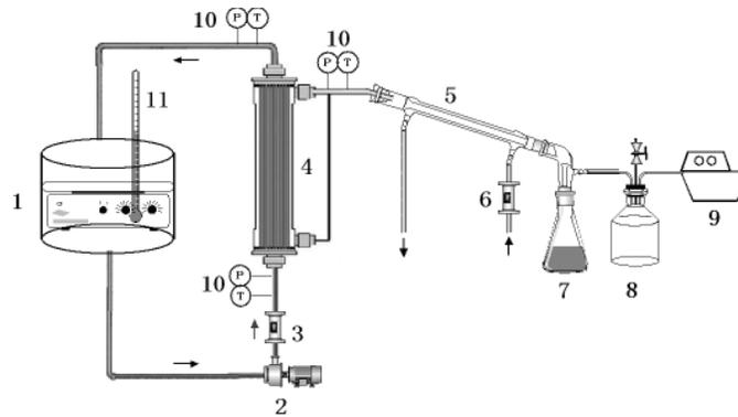
1: thermostat water bath; 2: magnetic pump; 3: flowmeter; 4: membrane module; 5: condenser pipe;
