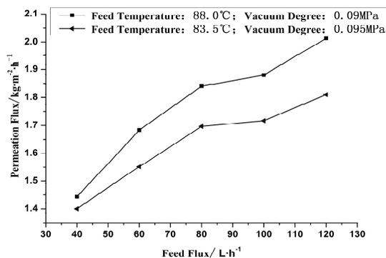
Fig.5 Influence of feed flux on permeation flux
