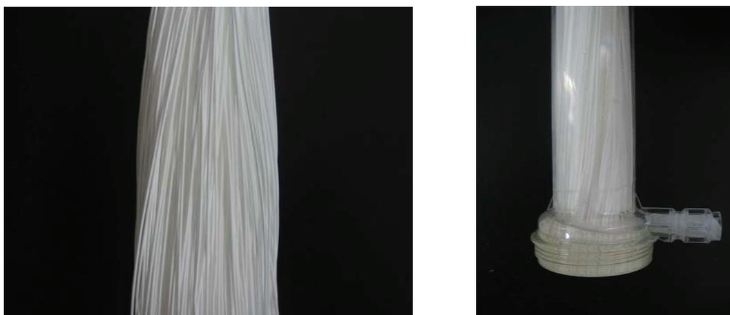
(a) PVDF membrane material (b) hollow fiber membrane module
