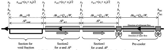
Figure 4: Estimation procedure for central vapor qualities in each section
