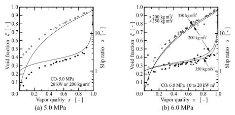
Figure 5: Experimental results on void fraction with present correlations
