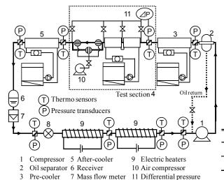
4 Test section 8 Expansion valve transducer Figure 1: Schematic diagram of an experimental refrigeration cycle
