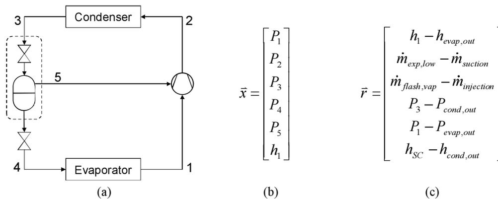
Figure 5: (a) Diagram of flash tank cycle, (b) vector of unknown variables, and (c) corresponding set of residual equations for the flash tank cycle
