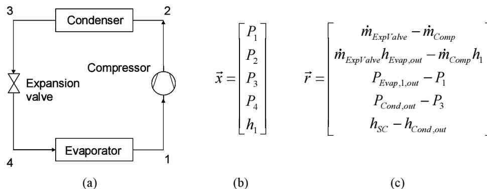
Figure 3: (a) Diagram of basic vapor compression system, (b) vector of unknown variables, and (c) corresponding set of residual equations for the baseline system
