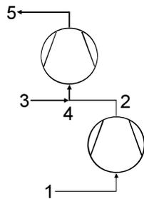
Figure 4: Diagram of a two stage vapor injection compressor model
