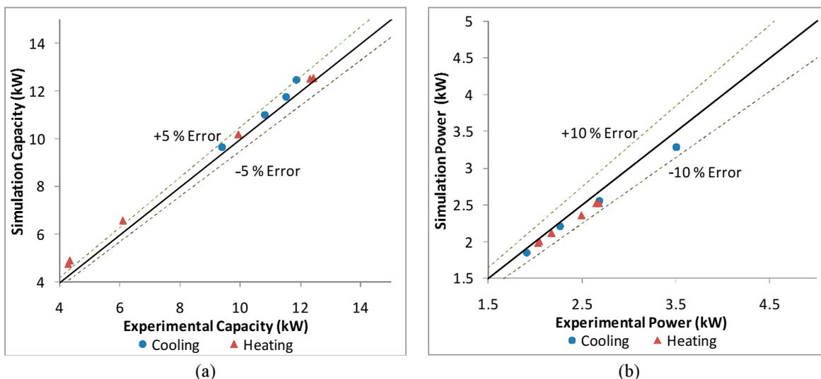
Figure 6: Baseline cycle validation results for (a) system capacity and (b) compressor power consumption
