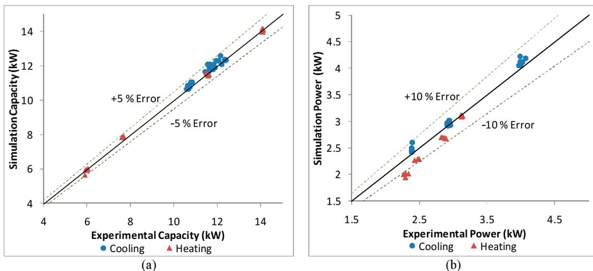
Figure 8: Flash tank cycle validation results for (a) system capacity and (b) compressor power consumption
