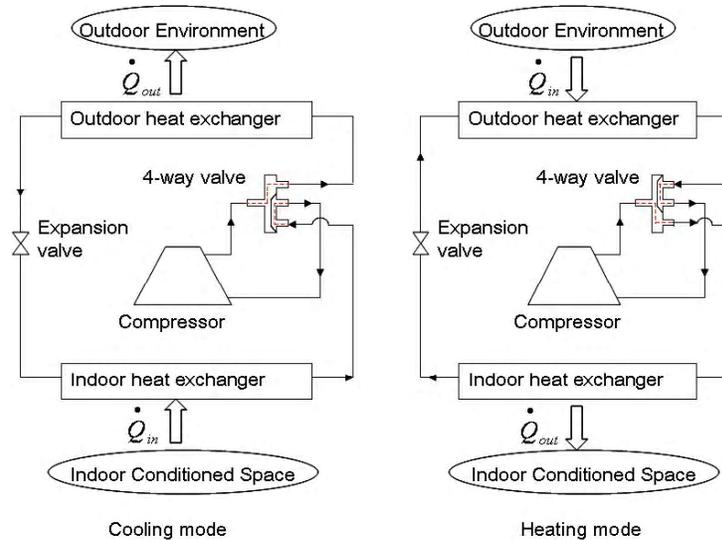
Figure 1: Diagram of a typical vapor compression heat pump
