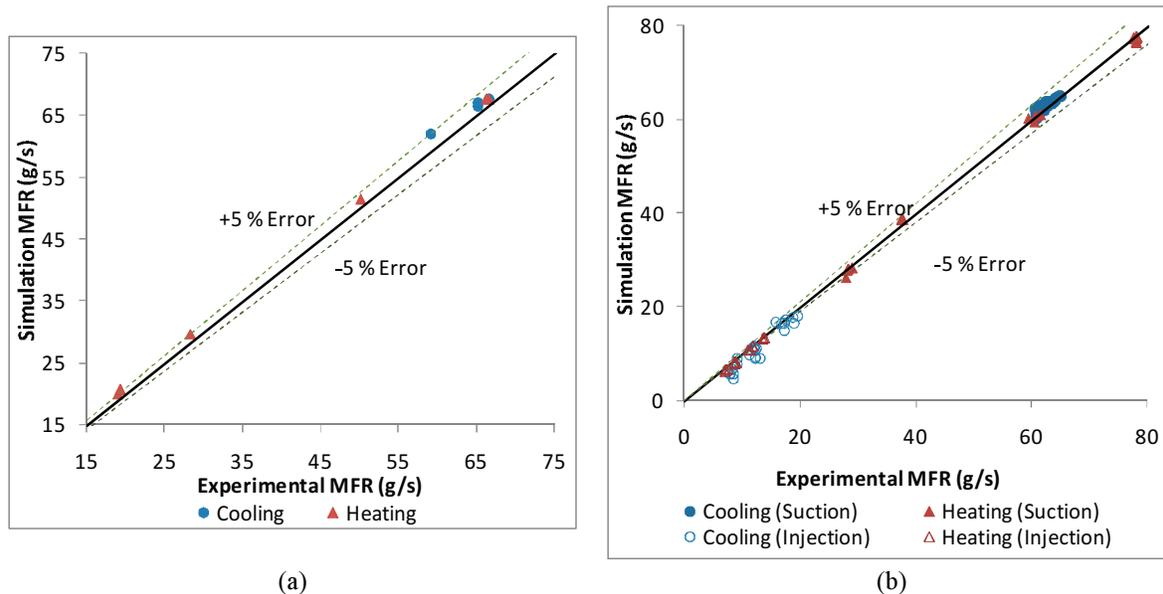
Figure 7: Mass flow rate results for the (a) baseline system and (b) flash tank cycle
