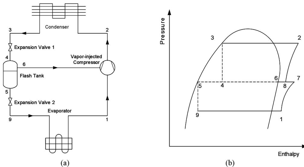
Figure 2: Diagram of a two-stage flash tank cycle
