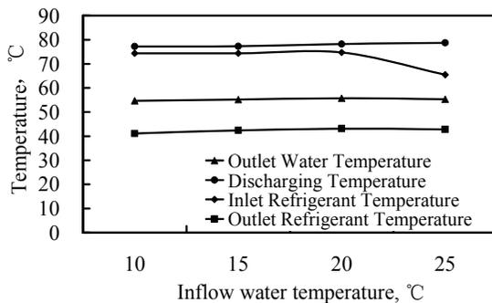
Figure 5: Experimental results of variable inflow water temperature
