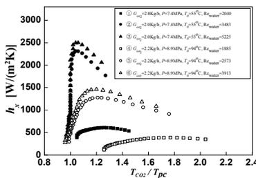
Figure 6: Local CO<sub>2</sub> heat transfer coefficient for various temperatures
