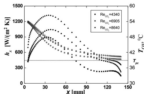
Figure 8:  $h(x)$  and  $T_{bulk}(x)$  for various  $G_{CO_2}$
