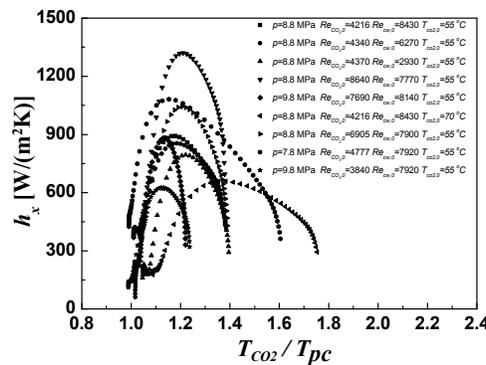
Figure 11: Local  $CO_2$  heat transfer coefficient for various  $CO_2$  temperatures
