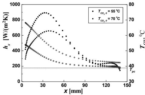
Figure 9:  $h(x)$  and  $T_{\text{bulk}}(x)$  for various  $T_{\text{in}}$
