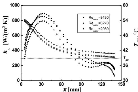
Figure 7:  $h(x)$  and  $T_{bulk}(x)$  for various  $G_{water}$
