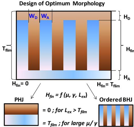
Fig 4. Design rules for fabricating the optimum morphology. The optimum fin width ( $W_{fin}$ ) and the fin height ( $H_{fin}$ ) height are determined as a function of the transport parameters.
