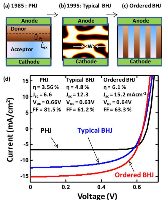
Fig. 1: Structure of the (a) PHJ, (b) typical BHJ and (c) ordered BHJ (OHJ) solar cell in the chronological order of development. (d) Comparison of I-V characteristics for various OPV geometry. The assumed model parameters are:  $L_{ex} = 20 \text{ nm}$ ,  $\mu_e = \mu_h = 10^{-3} \text{ cm}^2 \text{ V}^{-1} \text{ s}^{-1}$ ,  $\gamma = 10^{-9} \text{ cm}^3 / \text{ s}$ ,  $G_o = 10^{22} \text{ cm}^{-3} / \text{ s}$  (uniform),  $T_{film} = 100 \text{ nm}$ .
