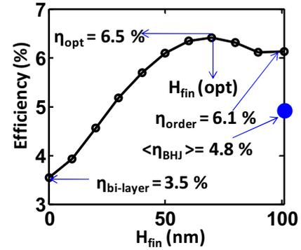
Fig. 5. Efficiency variation of FIN-OPV (Fig. 4) is plotted for the various fin heights. The fin width is kept fixed to the value of  $W_{fin} = 1.5L_{ex}$ . We find optimum fin height to be  $H_{fin}(opt) \sim T_{film} - \xi L_{ex}$ , where  $\xi$  is a number in the range ( $1 < \xi < 2$ ).
