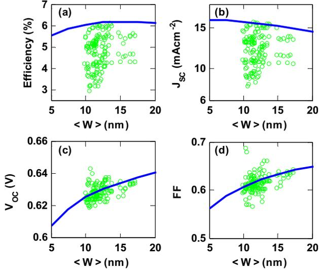
**Fig. 2: Performance comparison of ordered and disordered BHJ solar cell. The performance matrices are (a) efficiency ( $\eta$ ), (b) short circuit current ( $J_{sc}$ ), (c) open circuit voltage ( $V_{oc}$ ), and (d) fill factor ( $FF$ ). Each scattered symbol corresponds to a particular random morphology with an average domain size  $\langle W \rangle$  (x-axis). Solid line represents the performance of ordered geometry with domain width in x-axis.**
