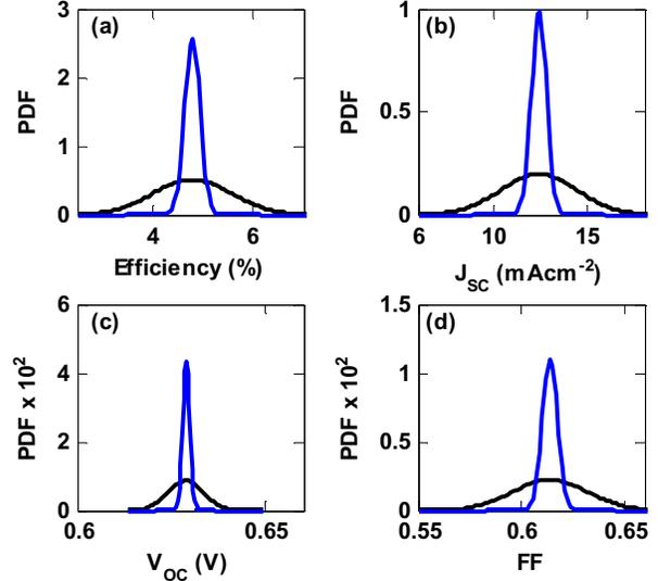
**Fig. 3: Probability density function (PDF) of the solar cell performance matrices ((a) efficiency ( $\eta$ ), (b) short circuit current ( $J_{sc}$ ), (c) open circuit voltage ( $V_{oc}$ ), and (d) fill factor ( $FF$ )). Variation in the performance arises from the structural randomness. Black solid curves are for devices with smaller active area (100nm x 100nm) and blue lines are for larger active area.**
