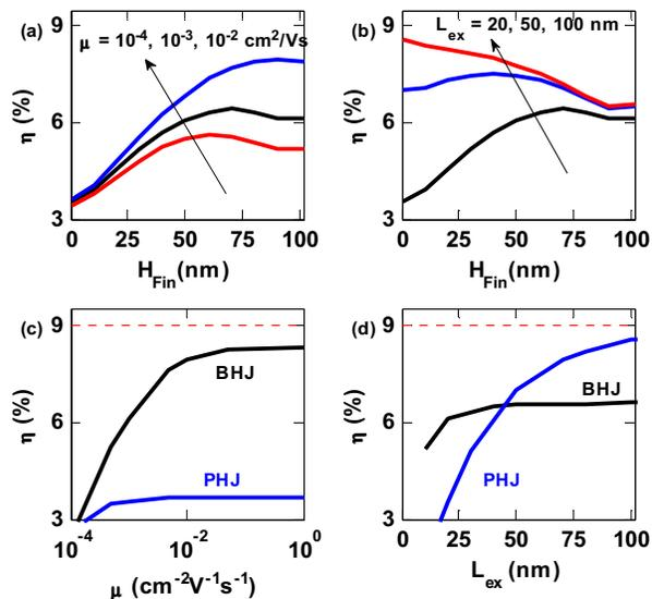
**Fig. 6. Efficiency variation with improved transport parameters. (a) Effect of carrier mobility and (b)  $L_{ex}$  on the FIN-OPV cell is shown. Efficiency improvement of both PHJ and ordered BHJ with respect to (c) mobility and (d) exciton diffusion length is plotted.**
