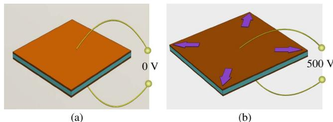
Fig. 1. Operation principle of dielectric elastomeric actuators. (a) Relaxed state. (b) Actuated through application of a voltage to the compliant electrodes.
