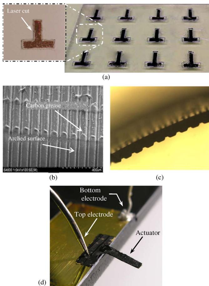
Fig. 9. (a) Batch-fabricated actuators. (b) SEM picture of the actuator showing corrugated surface. (c) Cross-sectional photograph of the actuator. (d) Mounted actuator.
