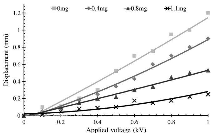
Fig. 12. Deflection versus applied voltage with different masses placed on the tip of the cantilever ( $l_1 = 20 \mu\text{m}$ ,  $l_2 = 70 \mu\text{m}$ ,  $t_1 = 40 \mu\text{m}$ , and  $t_2 = 70 \mu\text{m}$ ).
