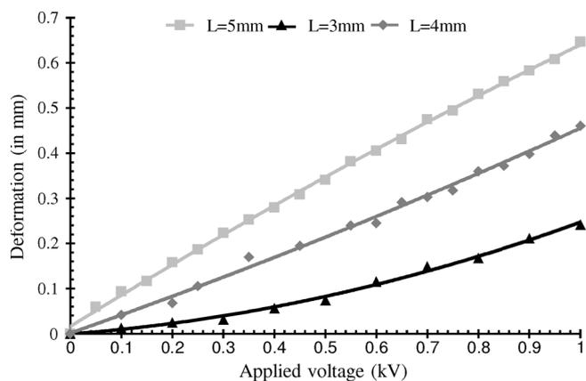
Fig. 10. Displacement versus applied voltage for actuators having 3-, 4-, and 5-mm lengths ( $l_1 = 20 \mu\text{m}$ ,  $l_2 = 70 \mu\text{m}$ ,  $t_1 = 40 \mu\text{m}$ , and  $t_2 = 100 \mu\text{m}$ ).
