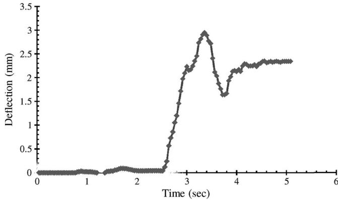
Fig. 13. Time response of the actuator when 1200 V was applied at 0.5 s.
