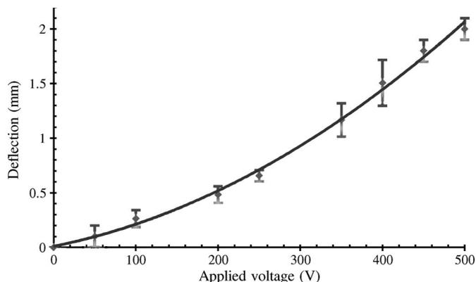
Fig. 11. Tip displacement versus applied voltage. The actuator movement was greatly enhanced by reducing the Young's modulus of the PDMS.
