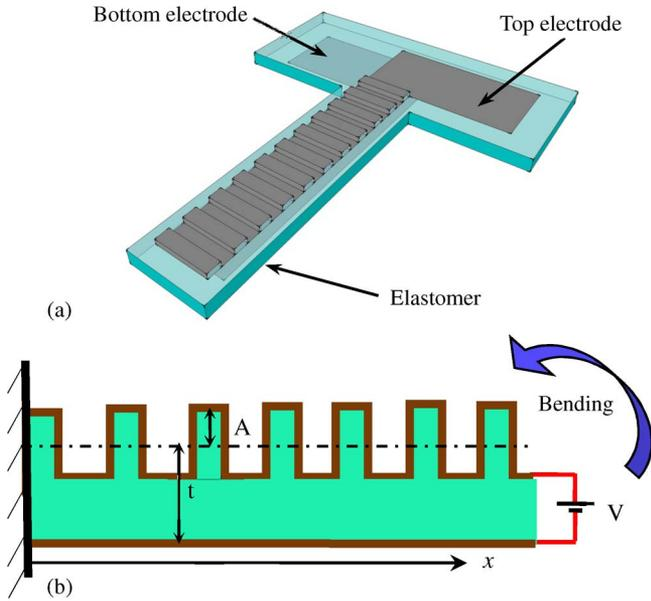
Fig. 2. (a) Three-dimensional schematic and (b) cross-sectional view of a single-layer elastomeric actuator with an asymmetric surface profile.
