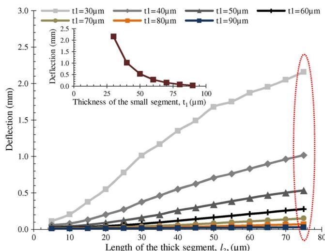
Fig. 6. Simulation results for asymmetric actuators showing tip deflection versus the length of the thick segment ( $t_1$  as the variable parameter). (Inset) Deflection versus the thickness of the thinner segment with other parameters kept constant (see the text).
