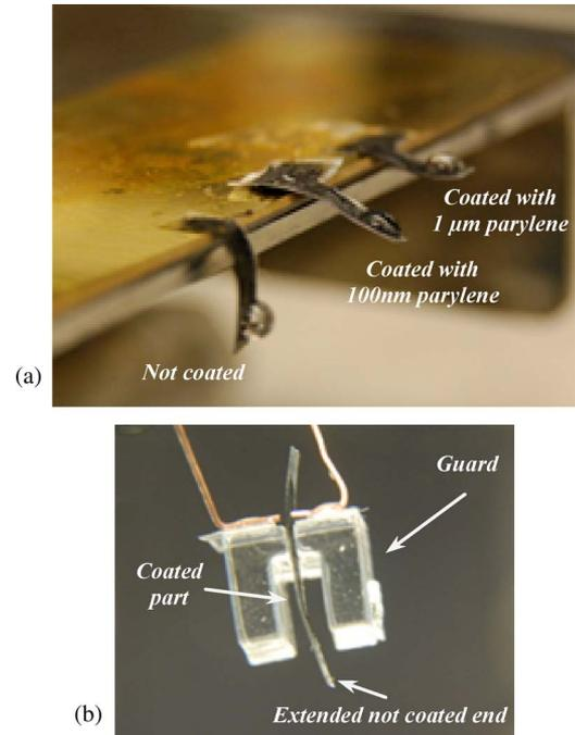
Fig. 14. Isolation of the elastomeric actuator. (a) Parylene coating increases the stiffness and degrades the performance, (b) enclosing the actuator in an acrylic guard.
