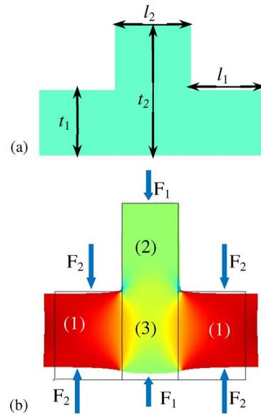
Fig. 3. Simplified structure of one element of the asymmetric actuator. (a) Without applied voltage. (b) With applied actuation voltage inducing a bending moment in the element.
