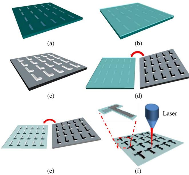
Fig. 8. Batch-scale fabrication process of the elastomeric actuators: (a) Etched silicon mold, (b) PDMS casting for the actuator, (c) PDMS stamp for the electrodes fabricated from an SU-8 mold, (d) stamping the electrodes on the actuator's flat surface, (e) stamping the electrodes on the corrugated surface, and (f) batch-scale separation with laser micromachining.
