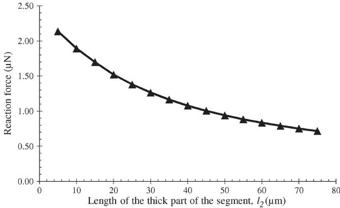
Fig. 7. Reaction force at the end of cantilever actuator versus the length of the thicker region with other parameters fixed (see the text).
