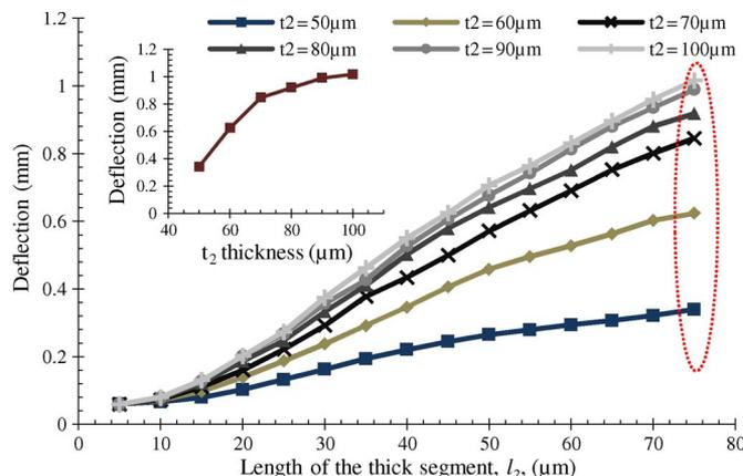
Fig. 5. Simulation results for asymmetric actuators showing tip deflection versus the length of the thick segment ( $t_2$  as the variable parameter). (Inset) Deflection versus the thickness of the thicker segment with other parameters kept constant (see the text).
