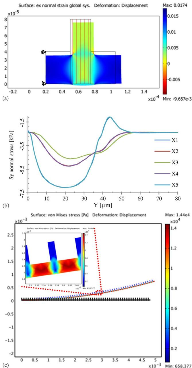
Fig. 4. Comsol simulation of a single element of the actuator. (a) Nonuniform displacement. (b) Normal stress along (shown by red lines) multiple cross sections. (c) Comsol simulation results for the 5-mm-long asymmetric actuator. Inset clearly shows nonuniform induced stress in the thicker segment.
