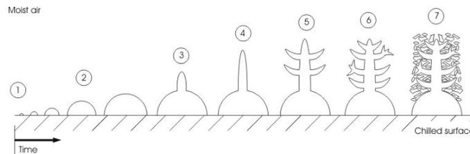
Figure 2. Schematic representation of the frost nucleation and growth processes (Tao et al., 1993)
