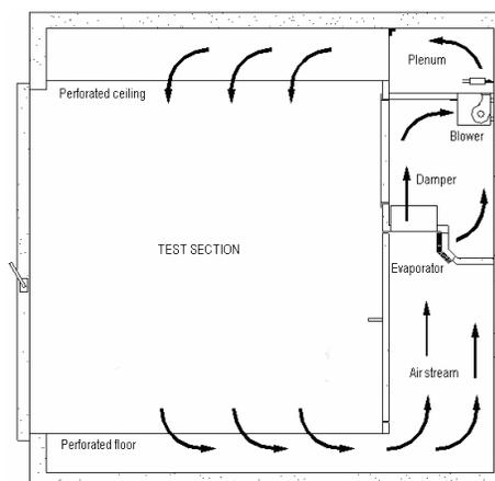
Figure 7. Schematic of the environmental chamber
