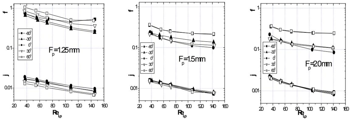
Fig. 5 Effect of inclination angle on  $j$  and  $f$  factors
