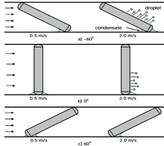
Fig. 4 Sketch of typical condensate drainage patterns
