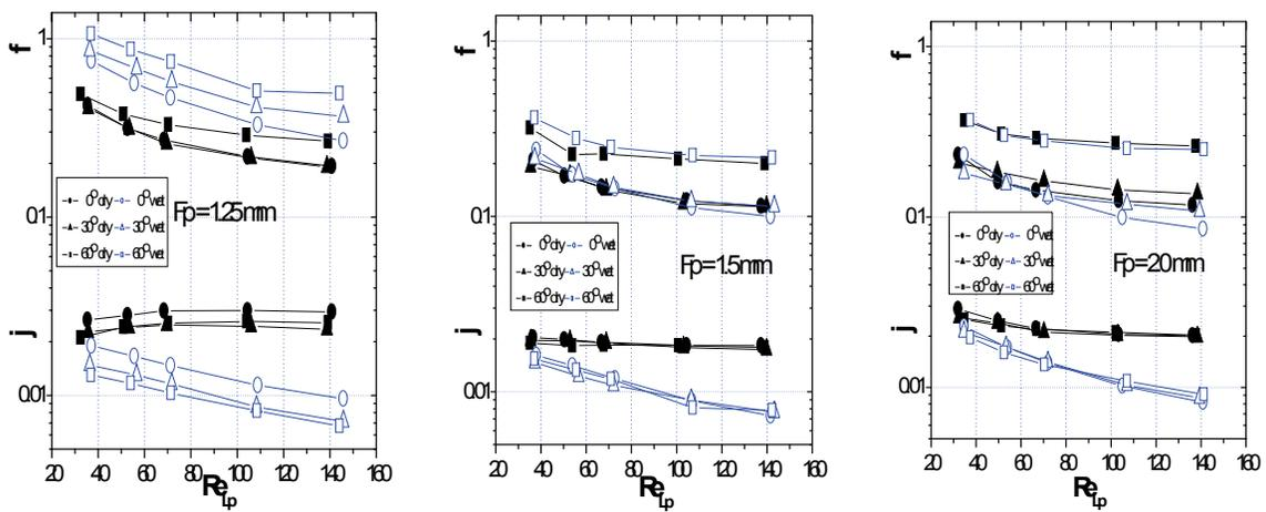
Fig. 7 Comparison of wet and dry  $j$  and  $f$  factors
