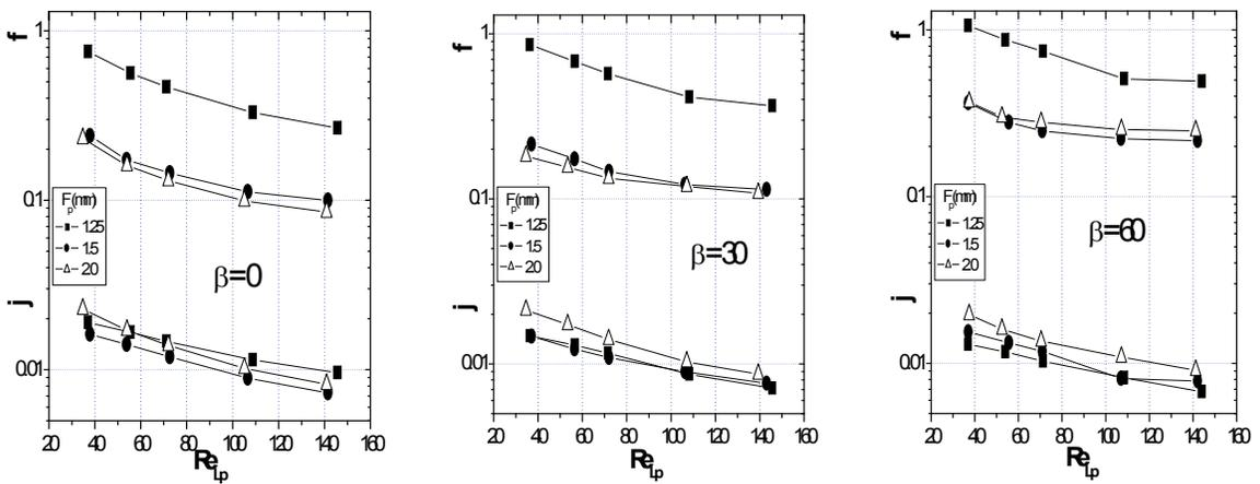
Fig. 6 Effect of fin pitch on  $j$  and  $f$  factors
