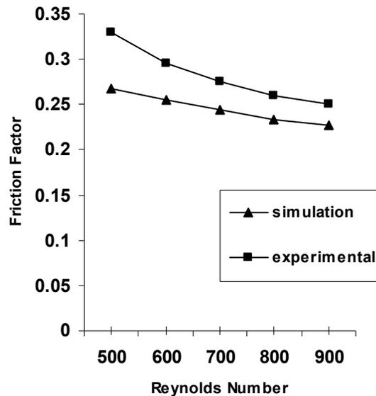
Figure 6. Comparison between predicted and experimental results for fanning friction factor for CC2.2-75 surface and air is the fluid.
