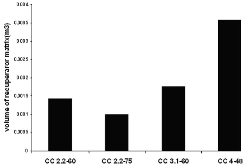
Figure 3. Results of design calculation, volume of the recuperator matrix for argon
