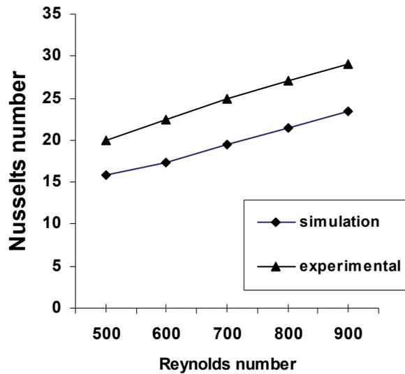
Figure 7. Comparison between predicted and experimental results for average Nusselt number for CC2.2-75 surface and air is the fluid.
