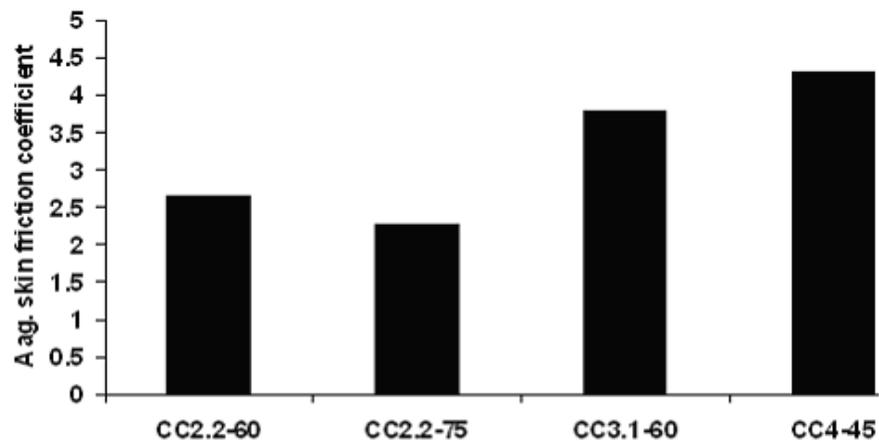
Figure 4. Results of CFD analysis, average skin friction coefficient for air
