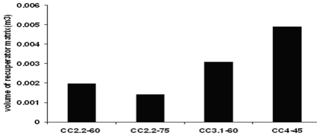
Figure 2. Results of design calculation, volume of the recuperator matrix for air
