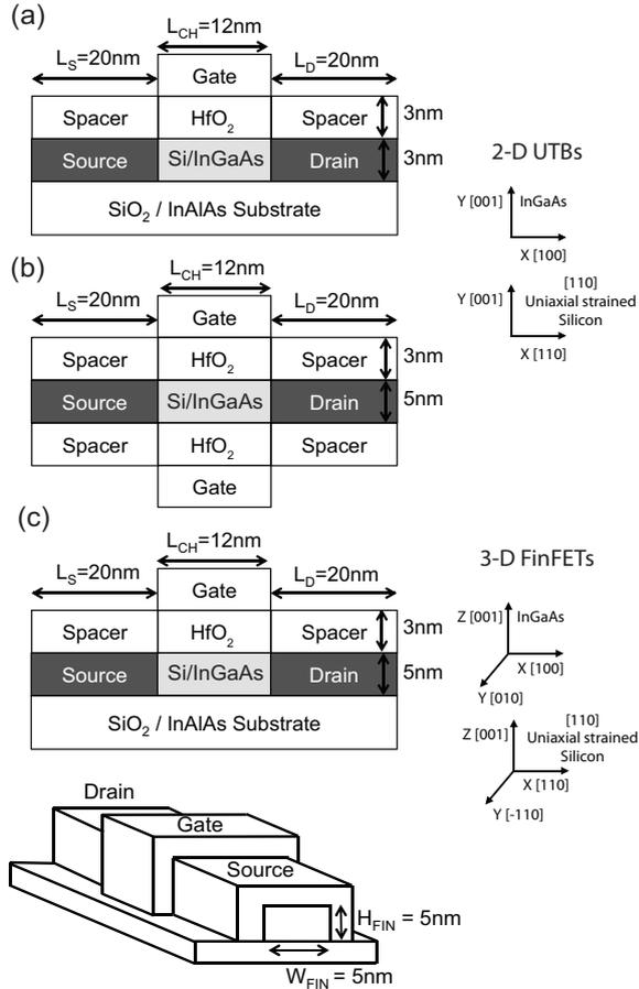
Fig. 1. Schematics of the simulated devices (a) Single-gate planar UTB FET (b) Double-gate planar UTB FET (c) 2-D and 3-D schematics of triple-gate FinFET.
