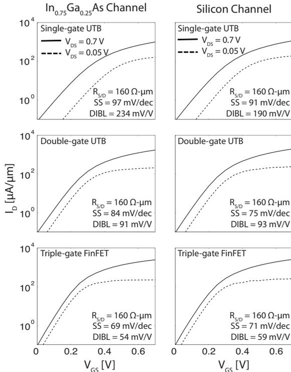
Fig. 4.  $I_D$ - $V_{GS}$  characteristics for the  $\text{In}_{0.75}\text{Ga}_{0.25}\text{As}$  and strained-Si FETs for two given drain voltage  $V_{DS} = 0.05\text{ V}$  and  $V_{DS} = 0.7\text{ V}$  with different gate voltages  $V_{GS}$  from 0.0 to 0.7 V (steps of 0.05 V) in semi-log scale.
