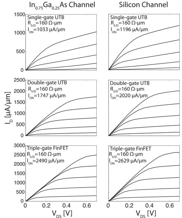
Fig. 5.  $I_D$ - $V_{DS}$  characteristics of the  $\text{In}_{0.75}\text{Ga}_{0.25}\text{As}$  and strained-Si FETs at six different gate voltages  $V_{GS} = 0.0\text{ V}$ ,  $0.3\text{ V}$ ,  $0.4\text{ V}$ ,  $0.5\text{ V}$ ,  $0.6\text{ V}$  and  $0.7\text{ V}$ .
