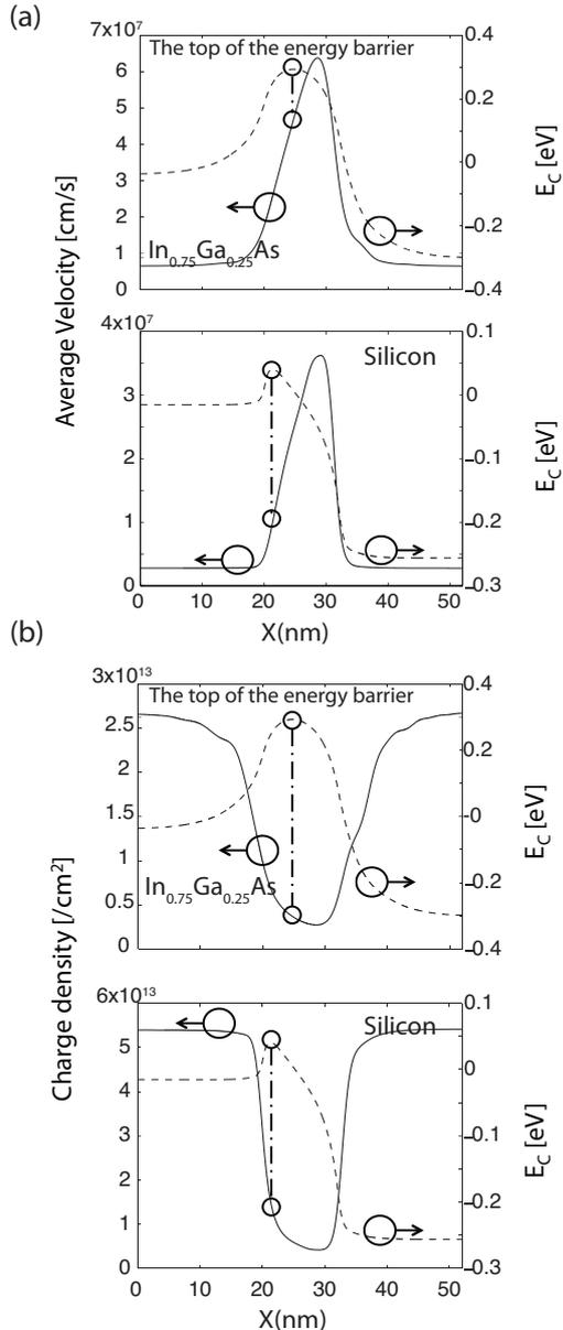
Fig. 7. (a) Ballistic injection velocity in the  $\text{In}_{0.75}\text{Ga}_{0.25}\text{As}$  and strained-Si double-/triple-gate FinFETs extracted at the top of the energy barrier (b) ON-state carrier density in the  $\text{In}_{0.75}\text{Ga}_{0.25}\text{As}$  and Si double-/triple-gate FinFETs extracted at the top of the energy barrier.
