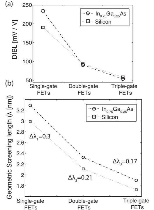
Fig. 6. (a)  $DIBL$  (b) Geometric screening length ( $\lambda$ ) of the  $\text{In}_{0.75}\text{Ga}_{0.25}\text{As}$  and strained-Si planar and non-planar FETs.
