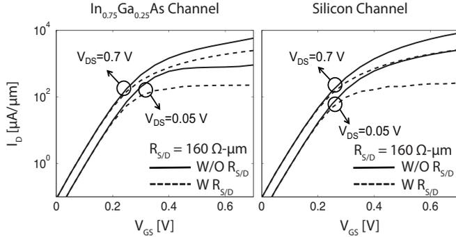
Fig. 3. Intrinsic (solid lines) and extrinsic (dashed lines)  $I_D$ - $V_{GS}$  characteristics of triple-gate FinFETs for (a)  $\text{In}_{0.75}\text{Ga}_{0.25}\text{As}$  and (b) strained-Si channels.
