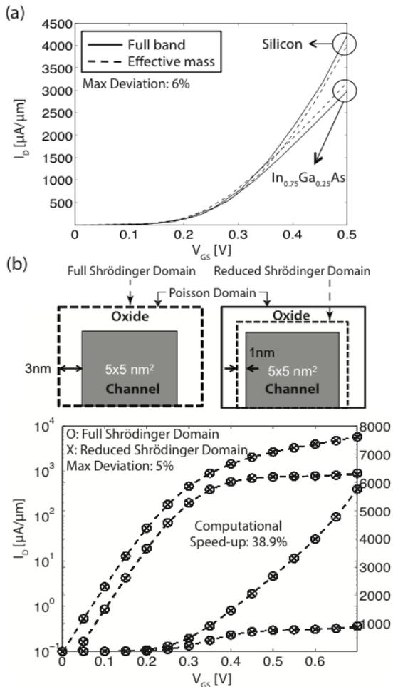
Fig. 2. (a) Basis reduction: comparison of the full-band (solid lines) and effective mass (dashed lines)  $I_D$ - $V_{GS}$  characteristics at  $V_{DS}=0.7$  V (b) Domain reduction: comparison of  $I_D$ - $V_{GS}$  characteristics of the strained-Si FinFET at  $V_{DS}=0.05$  V and  $V_{DS}=0.7$  V simulated using the entire Fin cross section (crosses) and reduced spatial domain that captures the wave function leakage (circles).
