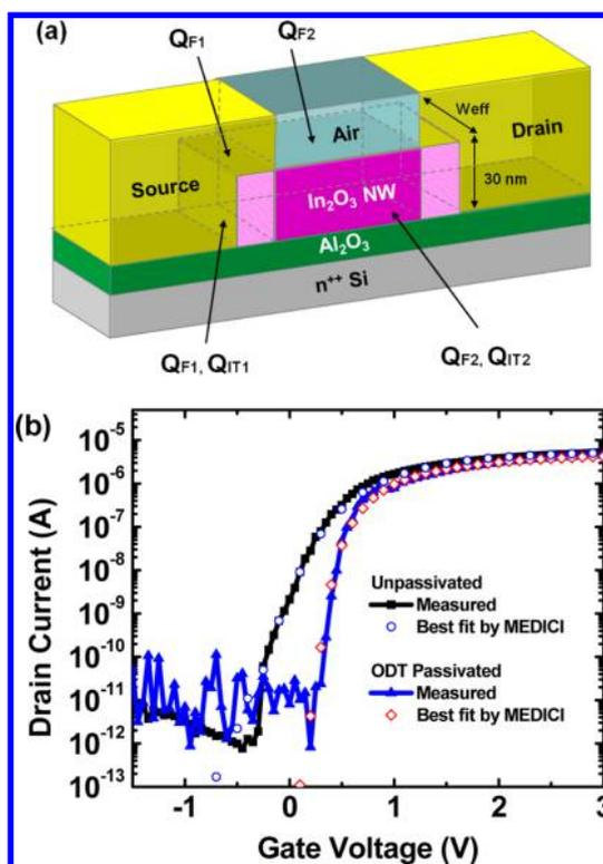
Figure 6. (a)  $\text{In}_2\text{O}_3$  nanowire transistor structure for MEDICI simulation, using rectangular geometry to approximate cylindrical nanowire region. The nanowire is divided into two regions, the region covered by the source and drain electrodes (dashed) and the region exposed to air defining the channel. (b) Transfer characteristics ( $I_{ds} - V_{gs}$ ) at  $V_{ds} = 0.5$  V from experimental data and best-fit MEDICI simulations before and after ODT passivation are shown.
