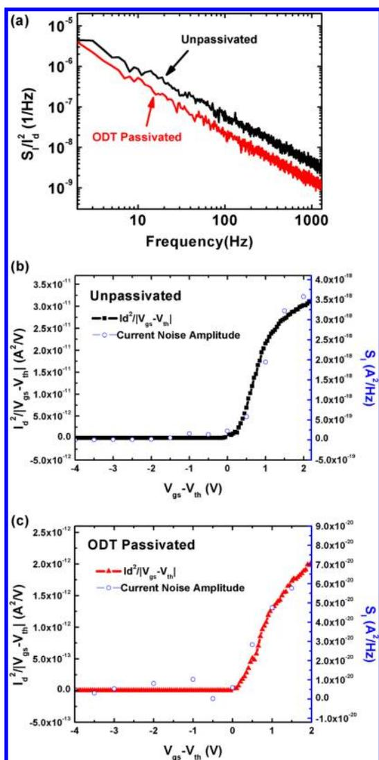
Figure 5. (a) Normalized current noise amplitude as a function of frequency for  $V_{gs} - V_{th} = 1.5$  V and  $V_{ds} = 0.5$  V before and after ODT passivation. Measured  $I_{ds}^2/|V_{gs} - V_{th}|$  and the amplitude of current noise spectrum (at 100 Hz) are plotted as a function of gate bias (b) before and (c) after ODT passivation for a fixed drain bias of 0.5 V.
