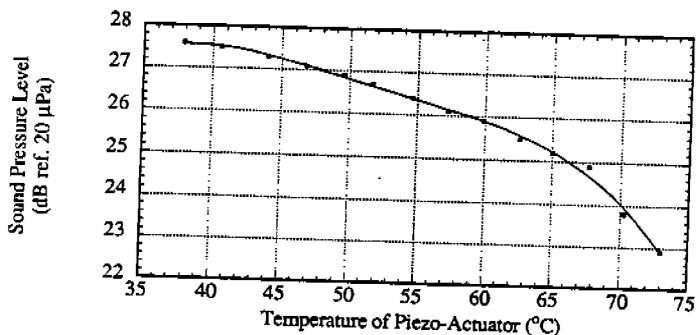
Figure 3. Effect of Temperature on the Performance of Piezo-Actuator.
