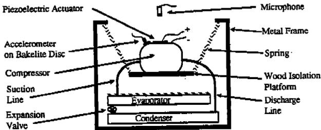
Figure 1. Compressor Load Stand.
