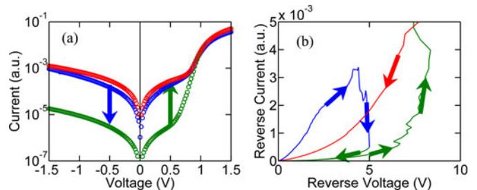
Fig. 7. (a) Initial dark IV characteristic (green) switches to the low  $I_{SH}$  state after voltage sweep (blue) and increases again after subsequent current sweep (red). (b) Abrupt switching transitions during voltage sweep showing the OFF transition (blue) and current sweep showing the ON transition (red).
