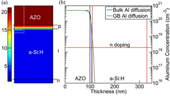
Fig. 4. (a) Two-dimensional simulation of Al diffusion during sputtering of top contact showing enhanced Al incorporation near the AZO grain boundary (dotted box). (b) One-dimensional plot of Al profiles show that the Al diffusion can overcome n-doping near grain boundary regions.
