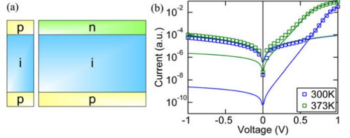
Fig. 3. (a) Separation of diode and shunt path allows simplification to 1-D structures. (b) One-dimensional simulations of shunt (dashed line) and diode (solid line) showing excellent match with dark  $IV$ -T data (symbols).
