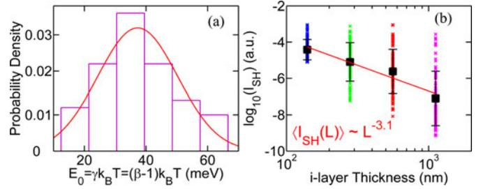
Fig. 5. (a) Extracted characteristic slope of band tails  $E_0$  is  $\sim 40$  meV for 61 devices, which is very close to the valence band tail slope in a-Si:H, as expected from the p-i-p shunt hypothesis. (b) Thickness dependence of the shunt current (at  $-2$  V) shows the inverse power law predicted by the SCL model; the crosses represent individual cells, and squares are geometric means with the error bars denoting the standard deviation.
