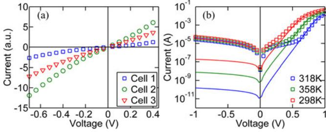
Fig. 1. (a) Symmetric non-Ohmic behavior about  $V = 0$  for three (symbols) nominally identical devices (scaled for clarity). (b) Temperature-dependent dark  $IV$  characteristics showing weak temperature dependence of  $I_{SH}$  (symbols, below 0.5 V), compared with the activated diode current (solid lines).
