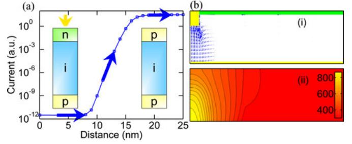
Fig. 9. (a) Simulation showing the change in reverse current at the location of shunt formation, as a function of distance of Al incorporation. As Al gets past the 20-nm n-layer, the current changes significantly (schematics in the inset). (b) Self-consistent simulations of the 2-D shunt structure at reverse bias of  $-7.5$  V, showing (i) localized shunt current and (ii) local heating effect (temperature scale in Kelvins) caused by the fast reverse sweep.
