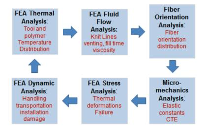
Figure 3 Composites molding simulation
