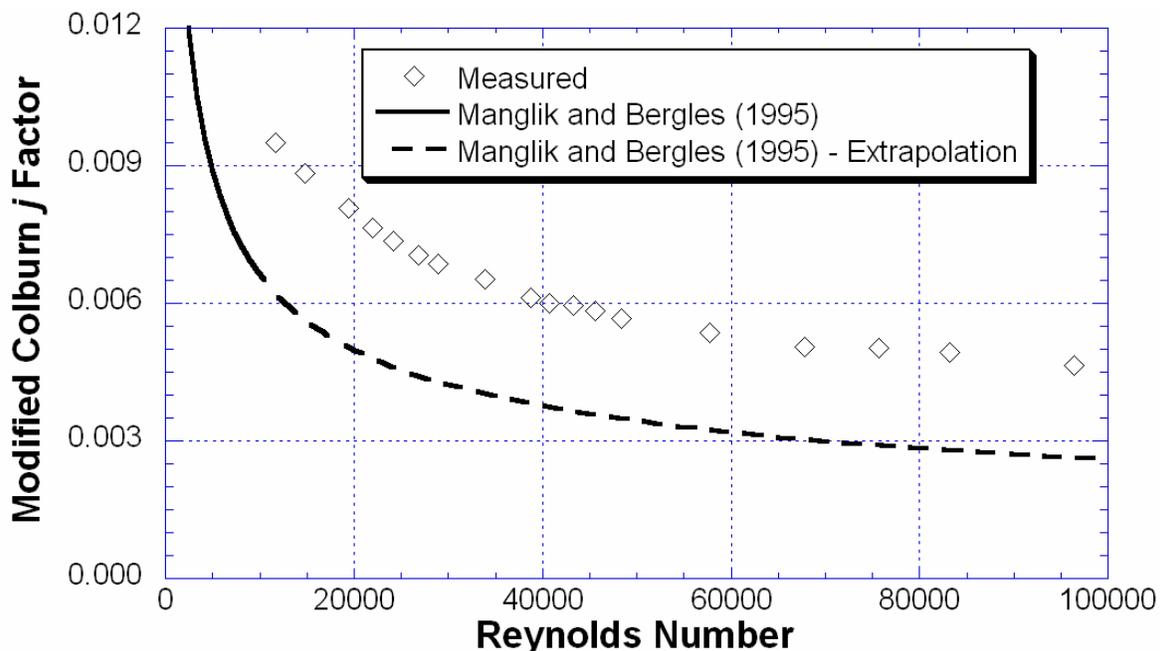
Figure 4. Modified Colburn  $j$  factor of the offset-strip fin array as a function of Reynolds number. The correlation of Manglik and Bergles (1995) is included for comparison.
