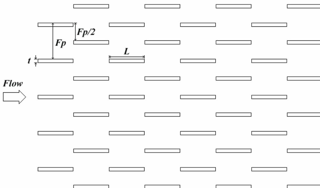
Figure 1. The geometry of the offset-strip fin array under investigation. The array height (into the page) was 146 mm,  $F_p = 25.4$  mm,  $L = 25.4$  mm, and  $t = 3.18$  mm.
