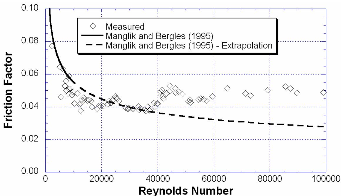
Figure 3. Fanning friction factor,  $f$ , of the offset-strip fin array as a function of Reynolds number. The correlation of Manglik and Bergles (1995) is included for comparison.
