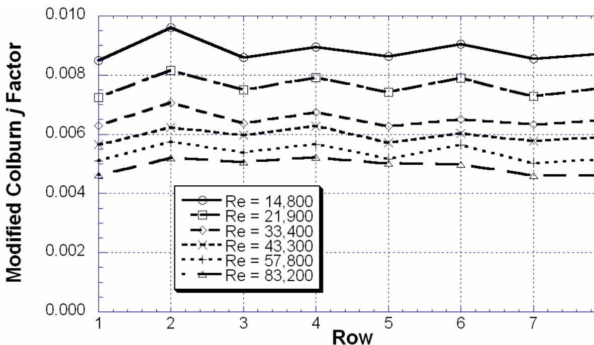
Figure 5. Row-by-row modified Colburn  $j$  factors at 6 different Reynolds numbers.
