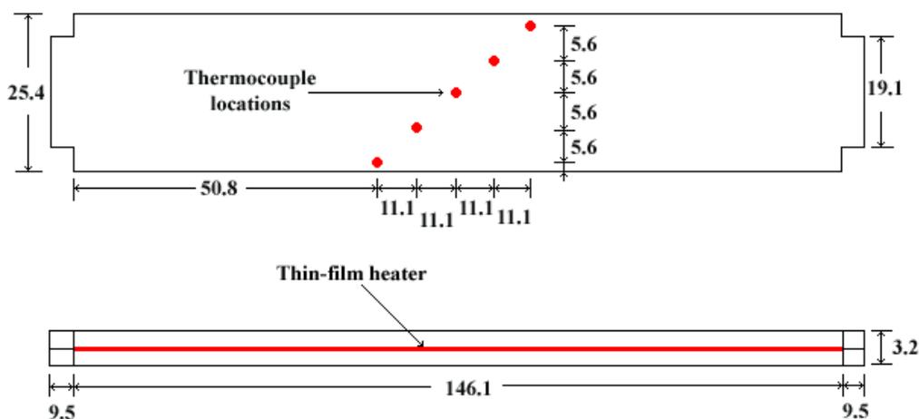
Figure 2. Geometry of the measurement fins. All dimensions are in mm.
