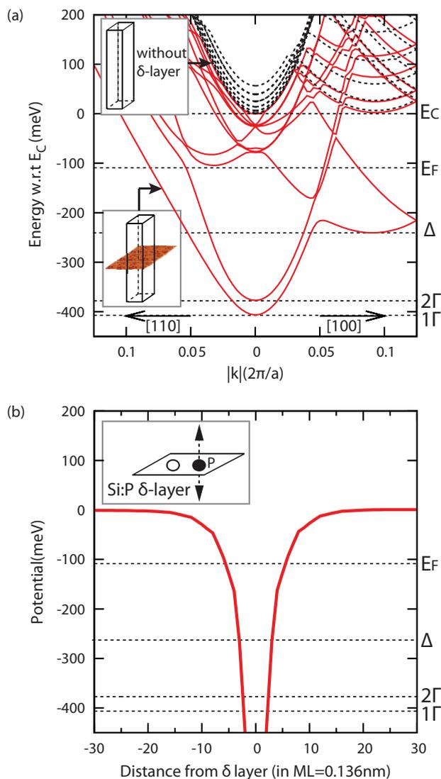
FIG. 3. (Color online) (a) Equilibrium band structure of an ideal ordered 1/4 ML Si:P  $\delta$ -doped layer at 4 K. The band structure of a pure silicon structure with the same dimension without the  $\delta$ -doped layer is plotted (dashed line) for comparison. (b) Potential profile plotted along confinement direction ([001]) passing through impurity site. The relative position of the valley minimum point and Fermi level with respect to the silicon conduction band minimum is indicated.
