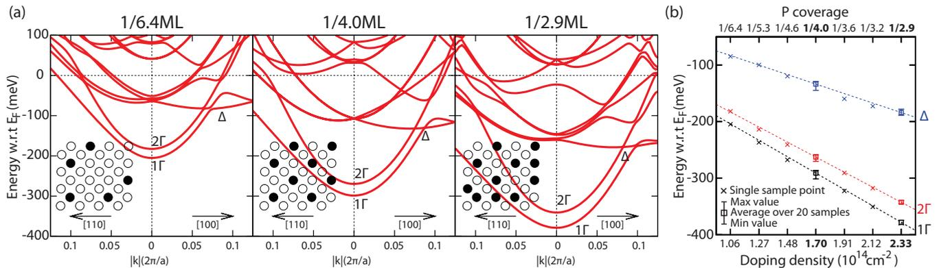
FIG. 6. (Color online) (a) Band structure results of 1/6.4, 1/4.0, and 1/2.9 ML  $\delta$ -doped layers. Inset in each band structure plot provides dopant placement used for the simulation. Due to odd number of dopants in 1/6.4 and 1/2.9 ML cases, unavoidable disorders are present. (b) Valley minimum values of different doping densities plotted with respect to the Fermi level. Statistical samples of 1/4.0 and 1/2.9 ML cases are plotted against other doping cases.
