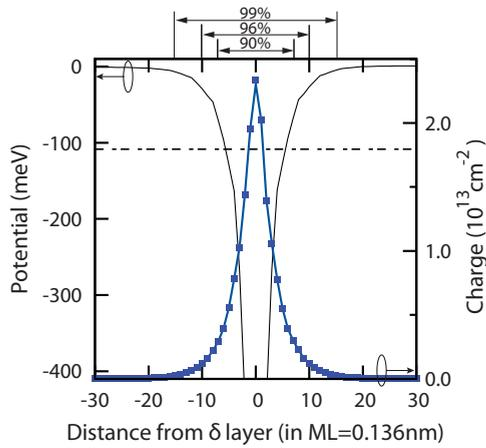
FIG. 5. (Color online) Charge profile of a perfectly ordered 1/4 ML Si:P  $\delta$ -doped layer at 4 K. 90%, 96%, and 99% of the charge is confined within 15 (2.03 nm), 21 (2.85 nm), and 31 (4.21 nm) ML, respectively. For reference, FWHM = 7 ML (0.81 nm) and it contains 66% of the charge.
