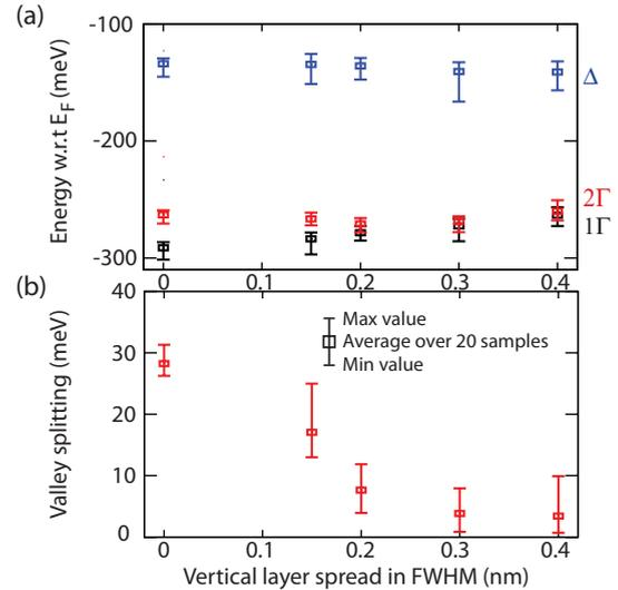
FIG. 10. (Color online) (a)  $1\Gamma$ ,  $2\Gamma$ , and  $\Delta$  valley minimum values are plotted with respect to the Fermi level vs vertical impurity segregation. Statistical samples of vertical segregation of dopant atoms with a nominal 1/4 ML doping is considered. (b) Valley splitting as a function of vertical segregation.
