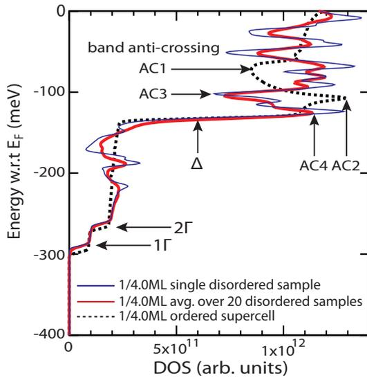
FIG. 9. (Color online) DOS comparison between ordered (dashed line) and disordered Si:P  $\delta$ -doped layers (solid lines). Fluctuations in DOS for ordered supercell is shown between AC1 and AC2 which is caused by band anticrossing labeled in Fig. 8(a). Similar fluctuation is also captured in disordered supercell between AC3 and AC4. For disordered cases, the DOS for single sample (blue) and the DOS averaged over 20 samples (red) are indicated.
