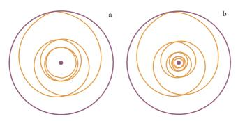
**Figure 7.** The trace of the light beam incident on the device at  $\phi_0 = 0.55\pi$  (a) p = 1.98, the beam makes about 10 turns; (b) p = 1.99, the beam makes 20 turns.
