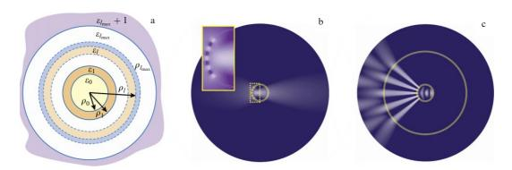
Figure 3. Concentric, cylindrical multilayered hyperlens. (a) Geometry of the layers. Five test sources with subwavelength spacing: (b) free-space radiation (the inset shows zoomed sources), (c) the same sources magnified by the hyperlens.
