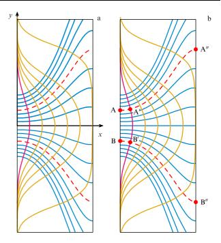
**Figure 1.** (a) Generating lines (red) and the matching orthogonal curvilinear coordinates. (b) Mapping the near-field virtual domain AA'B'B onto a material domain AA"B"B (with a scaling transformation).
