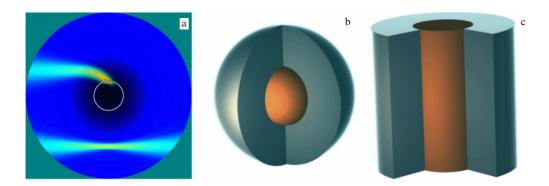
Figure 5. (a) A simulated light beam completely captured by the light absorber. The other beam propagares below, missing the device. (b, c) Schematic cross-section of light concentrators using all-dielectric designs. The center core is made of a strong light absorber, and the outer cladding is made of a dielectric material with a graded refractive index: (b) spherical design and (c) cylindrical design.
