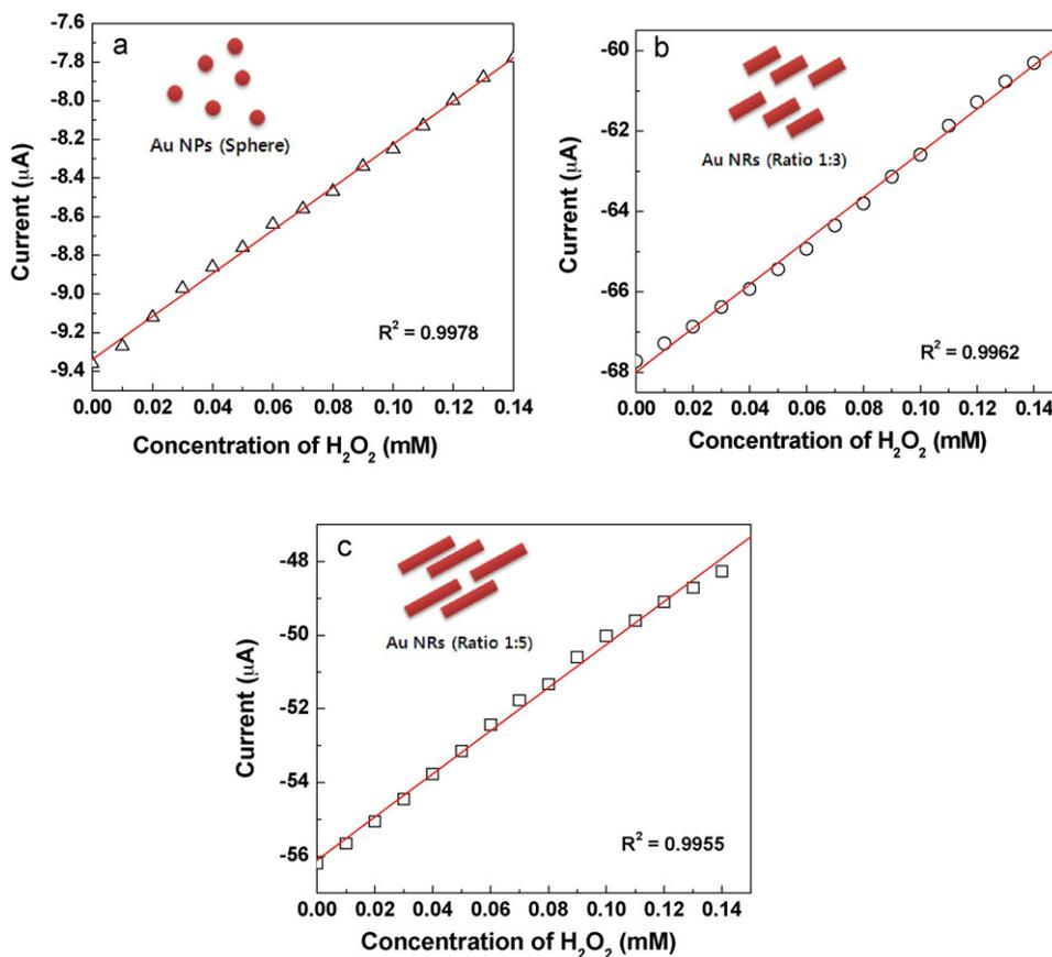
**Fig. 5.** Amperometric responses of enzyme-free biosensors for the detection of hydrogen peroxide in PBS (0.05 M, pH 5) containing 10 mM  $[\text{Fe}(\text{CN})_6]^{3-/4-}$  at an applied potential of 200 mV with successive additions of 0.01 mM hydrogen peroxide. (a) Au NS-based, (b) Au NR (1:3)-based, and (c) Au NR (1:5)-based biosensors, separately.
