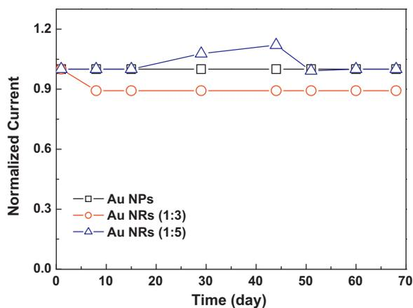
**Fig. 6.** Stability test of Au nanocrystal-based enzyme-free biosensors over 68 days in the PBS (0.05 M, pH 5) containing 10 mM  $[\text{Fe}(\text{CN})_6]^{3-/4-}$  at 200 mV to 0.33 mM hydrogen peroxide.
