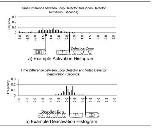
Figure 4-4. Example Histograms of Video Detection Timing Errors
