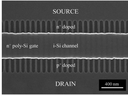
Fig. 1. Scanning electron microscope image of a NW-TFET array with a nominal wire pitch of 100 nm and wire width of  $\sim 20$  nm. An intrinsic Si channel region is preserved under the 500-nm-wide poly-Si gate and  $n^+$ - and  $p^+$ -regions were formed through ion implantation and RTA, ELA, and LT-RTA activation processes.
