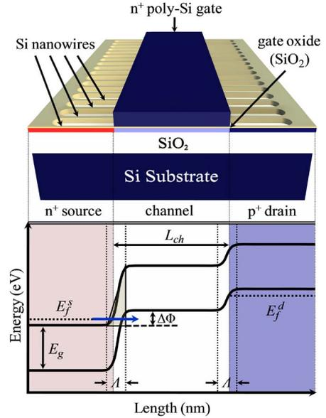
Fig. 2. Schematic representation of (top) the fabricated Si NW-TFET arrays with a cross-sectional slice of one of the NWs, showing the  $n^+$  source,  $i$ -Si channel, and  $p^+$  drain segments. (Bottom) The band diagram projection illustrates the hole current flow responsible for the p-branch tunneling characteristics when the valence band in the channel is above the conduction band edge in the source.
