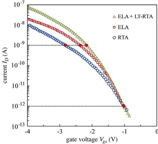
Fig. 4. Transfer characteristics shifted in  $V_{gs}$  to align the p-branches of RTA, ELA, and ELA + LT-RTA annealed NW-TFET devices at  $I_{OFF} = 10^{-12}$  A. (Dotted lines and large dots) The extraction points for  $S_{avg}$  over three orders magnitude change in  $I_D$ .
