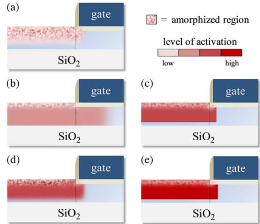
Fig. 5. Cross-sectional schematics depicting the expected relative levels of activation and dopant profile smearing at the source/channel junction under the gate for the activation conditions described in this paper, including: (a) as-implanted; (b) 1000 °C spike RTA; (c) 650 °C SPER only; (d) ELA only; and (e) ELA + 650 °C LT-RTA.
