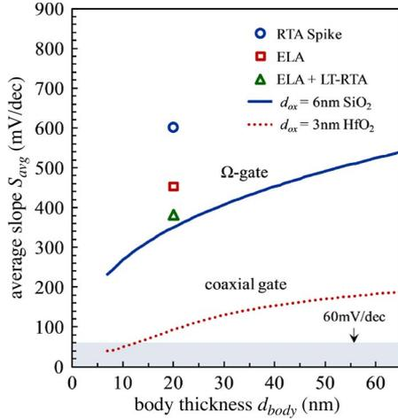
Fig. 6. Simulation curves, showing how  $S_{avg}$  over 3 orders magnitude change in  $I_D$  scales with  $d_{body}$ , are plotted together with experimentally extracted values of  $S_{avg}$  for RTA, ELA, and ELA + LT-RTA. Aggressively scaled NW-TFETs with  $d_{ox} = 3$  nm ( $\text{HfO}_2$ ) show the potential for sub-60 mV/dec operation for  $d_{body} < 13$  nm.
