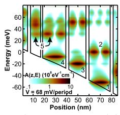
FIG. 2. (Color online) Calculated conduction band profile (line) and contour plot of the energy and spatially resolved spectral function A(z,E) at vanishing in-plane momentum in the proposed QCL at the threshold bias voltage of 68 mV per period and a lattice temperature of 100 K. The zero in energy marks the chemical potential of the source.
