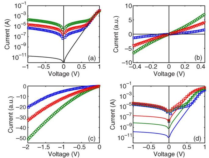
Fig. 1. (a) Dark IV characteristics of three nominally identical cells (symbols), compared to simulated IV (solid line). The (b) symmetry and (c) nonlinearity of the leakage current for the same three devices (current values are scaled for clarity). (d) Temperature-dependent dark IV of one of the devices (symbols), at 45 °C, 85 °C, and 120 °C, compared to simulations (solid lines).
