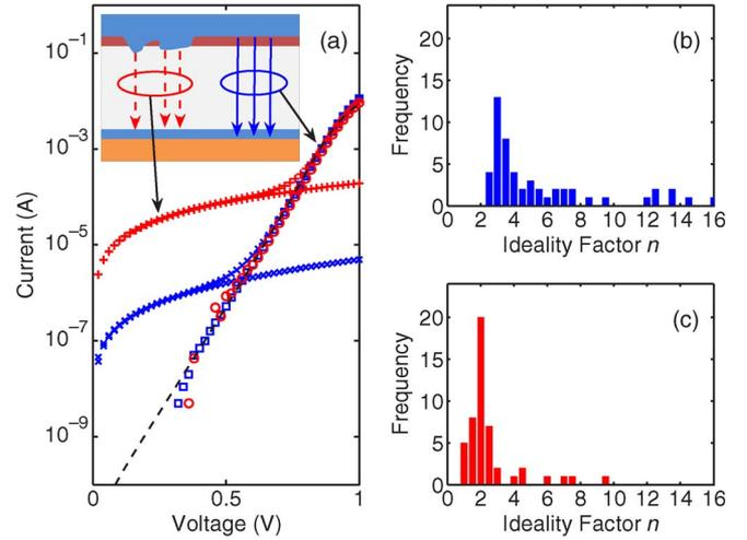
Fig. 3. (a) Plot showing that the cleaned  $IV$  (circles and squares), obtained by subtracting off the symmetric shunt in two devices (crosses and pluses), shows the expected exponential behavior. Histograms compare the spread of extracted ideality factor  $n$  (using  $n = q(V_2 - V_1)/k_B T \ln(I_2/I_1)$ , with  $V_2 = 0.7$  and  $V_1 = 0.4$ ) (b) before and (c) after removing the shunt component.
